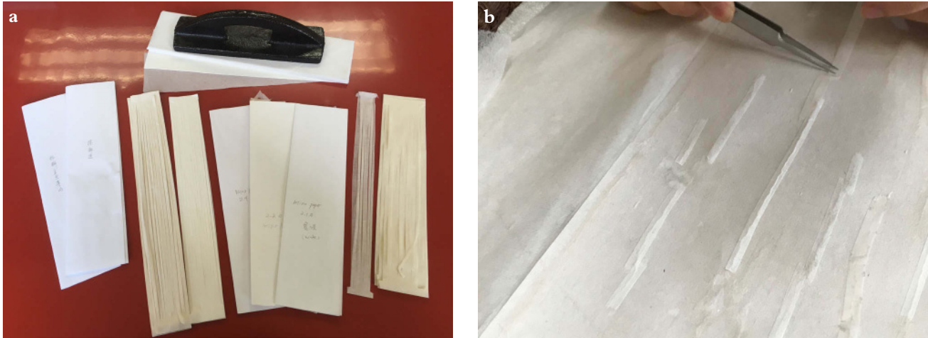
Fig. 11. (a) Chinese xuan paper and Japanese mino paper used for strip reinforcements. (b) Application of strip reinforcements.
