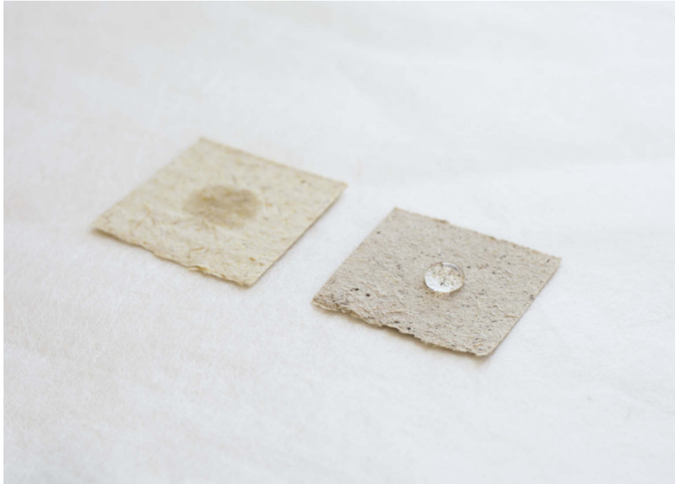
Fig. 9. Wettability testing on paper samples that have been externally size with 2% gelatin solution (right) and unsized (left)
