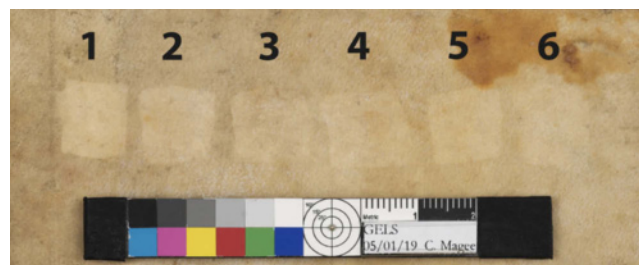
Fig. 12. Six gels were used in the experimental cleaning of a 16th-century parchment book cover. The numbers by the cleaned areas in the image correspond to the number of the gels in table 1. Image courtesy of the Walters Art Museum, Baltimore.
