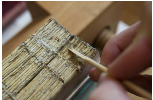
Fig. 11. The adhesive could be removed with a wooden spatula after becoming sufficiently softened.
