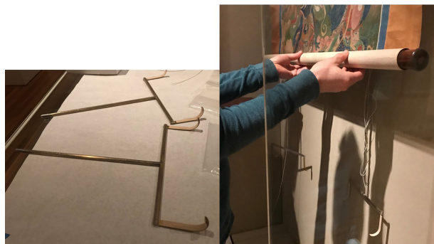
Fig. 26. Left: Metal supporting J-hooks. Right: The J-hooks are behind the hanging scroll.
