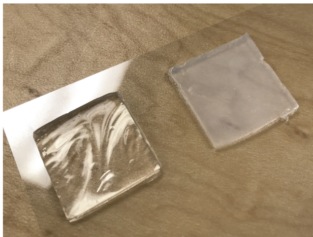
Fig. 5. Gellan gum made with DI water (left) vs. with 3% citric acid (right).
