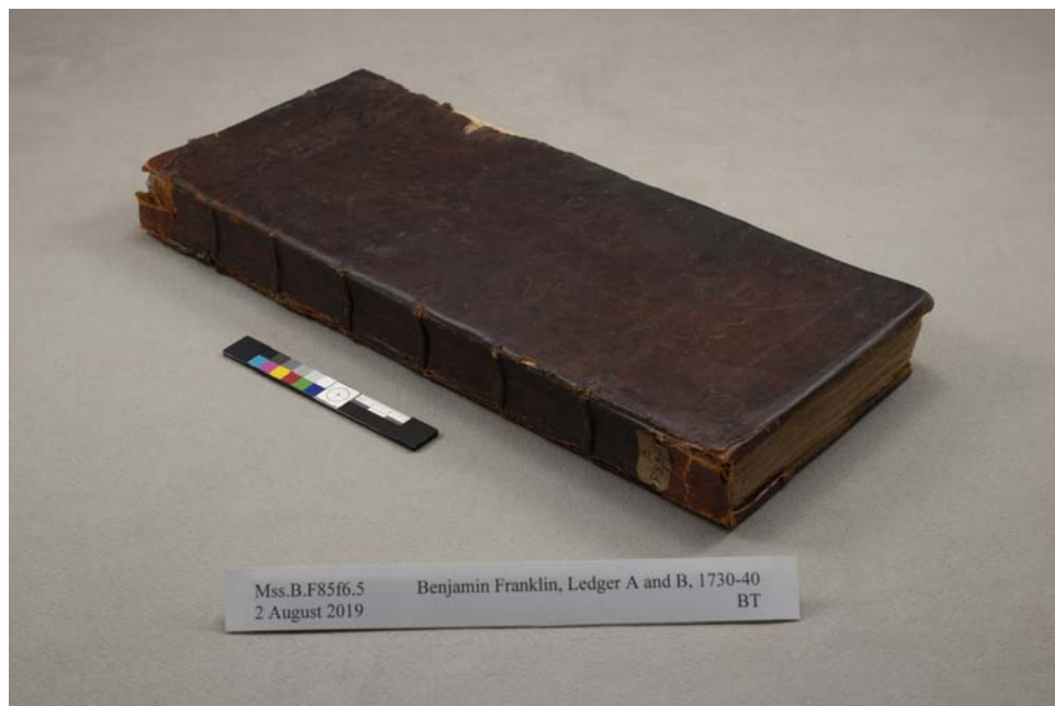
Fig. 38. By the time Ledger A and B was treated again in 2019, the vegetable-tanned leather Carol Rugh had used to repair its endcaps was weak, red, powdery, and torn. There was also new damage to the leather over the joints and front board. Benjamin Franklin, Ledger A and B, 1730–1740, Ms.B.F85.f6.5, American Philosophical Society.
