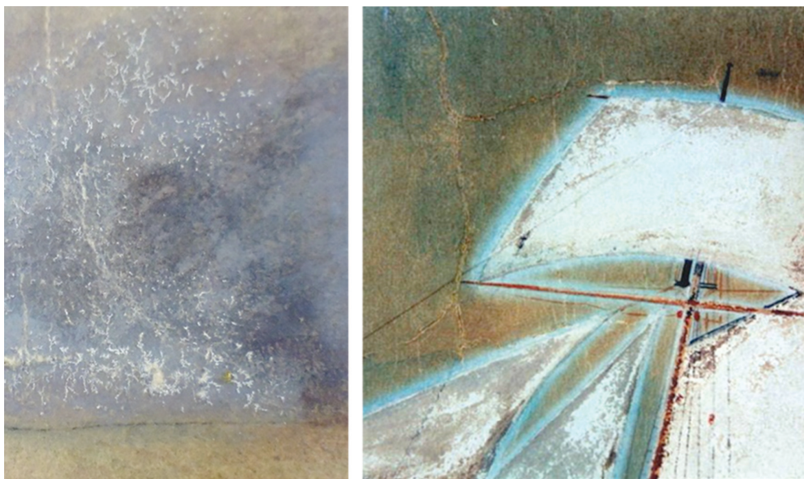
Fig. 1. Left : Detail of General View of St. Mary's Cathedral, Iona with sulfate salt efflorescence visible as needle-like blooms on the painting's surface. Right : Zinc sulfate salts have formed and dissolved into the paper, slowing the rate of paper discoloration and creating a pale halo. From Singer and Liddie (2005).
