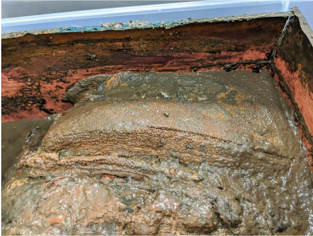
Fig. 3. The paper-based items in the time capsule had been soaking in acidic water. Although they retained vestiges of their original shape, the paper was soft and mushy, having lost all structure. Courtesy of Nicole Royal.
