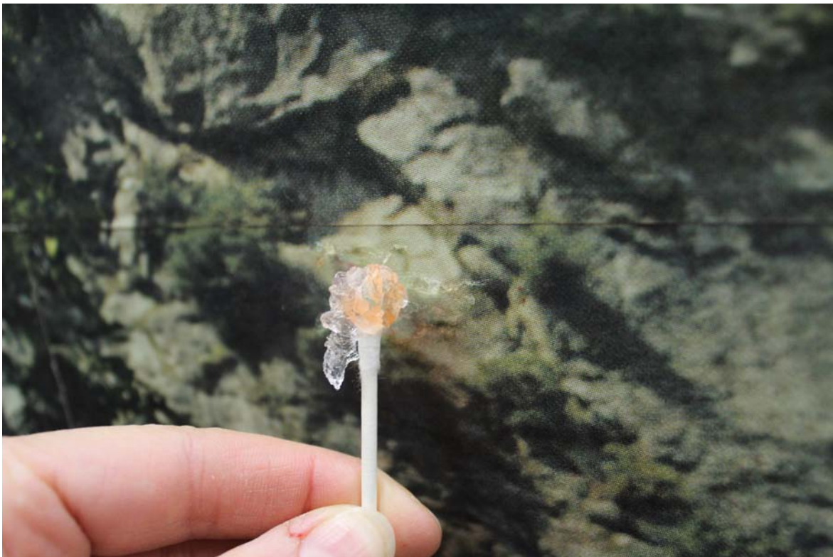
Fig. 7. Laponite on a cotton swab showing products of staining absorbed by poultice.
