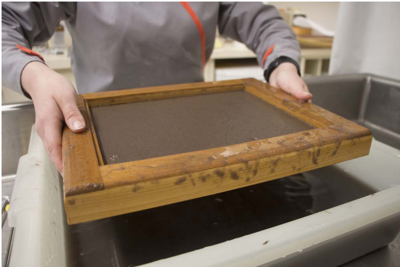
Fig. 6. Small sheets of paper were casted with the paper pulp mix and dried on a wooden board.
