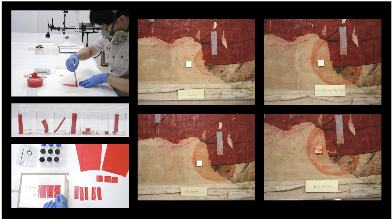
Fig. 5. Preliminary paint sample preparation and dissolving tests with different solvents.
