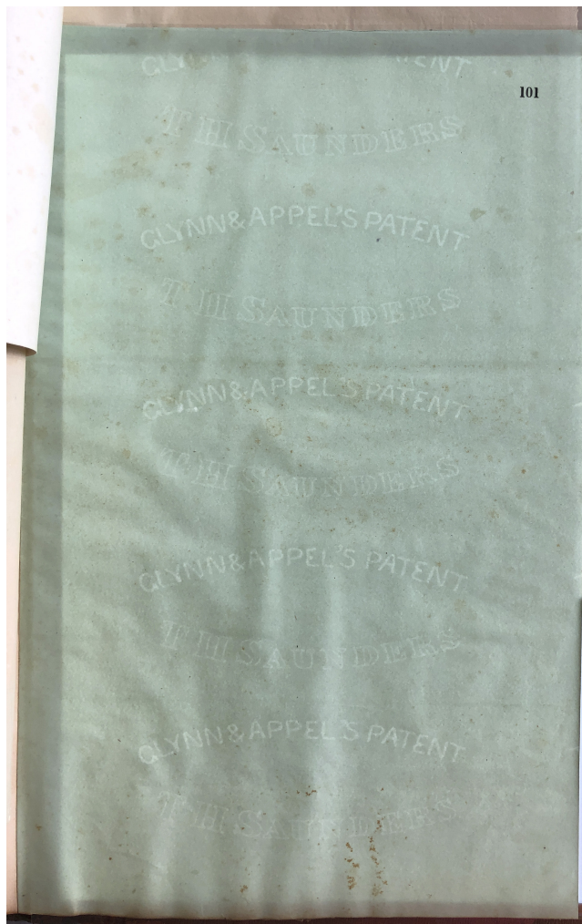
Fig. 4. Transmitted light photograph of Glynn & Appel's Patent security paper, sample 103. From Illustrations of the British Paper Manufacture , Queen's University, W.D. Jordan Rare Books and Special Collections, Rare Books Collection, FF TS1105 .S2.
