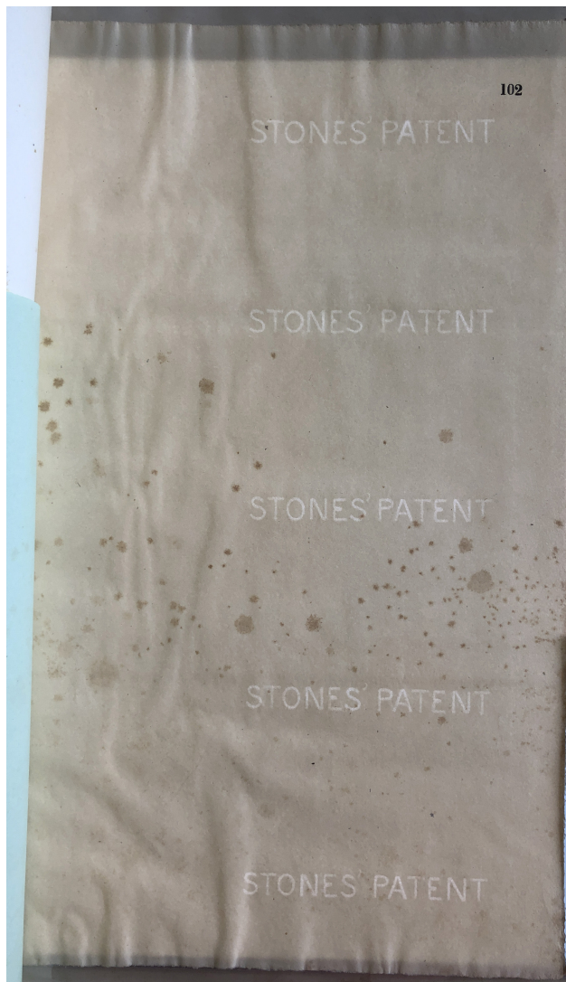
Fig. 5. Transmitted light photograph of Stones' Patent security paper, sample 102. From Illustrations of the British Paper Manufacture , Queen's University, W.D. Jordan Rare Books and Special Collections, Rare Books Collection, FF TS1105 .S2.
