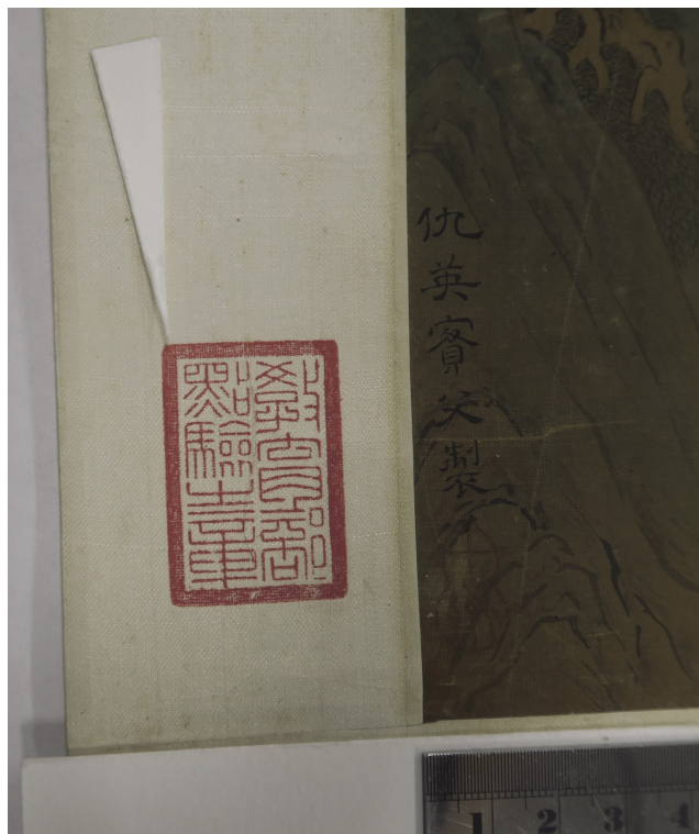
Fig. 10. Testing the stability of the red seal at the painting and border.
