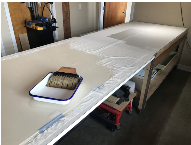
Fig. 10. Wetting out the cotton muslin with water.
