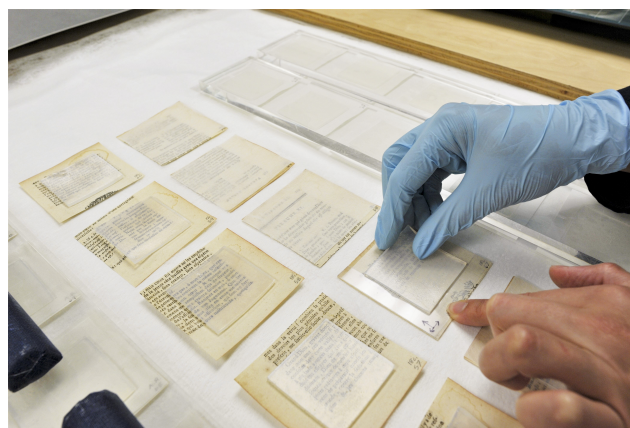
Fig. 1. Detail of experiment setup highlighting gel application, using a rigid polyester jig, on paper samples directly and with interleaving.
