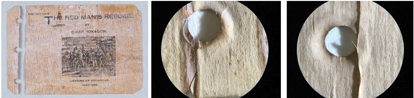
Fig. 8. The combination of vertical lenticels and the birch bark page flexing at the oversewing leads to splits in the page, as seen in the front cover of The Red Man's Rebuke (Special Collections Research Center, University of Michigan Library). Photomicrographs (15x magnification) show punched holes and a broken area within a lenticel of The Red Man's Greeting (AC85 P7565 893r, Houghton Library, Harvard University).
