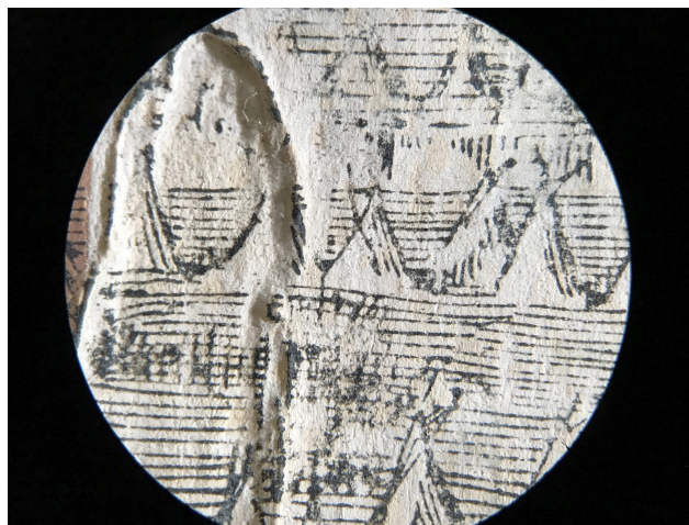
Fig. 2. Photomicrograph (15x magnification) of The Red Man's Greeting (AC85 P7565 893r, Houghton Library, Harvard University). An example of printing where the text sits only on the highest points due to the uneven surface.
