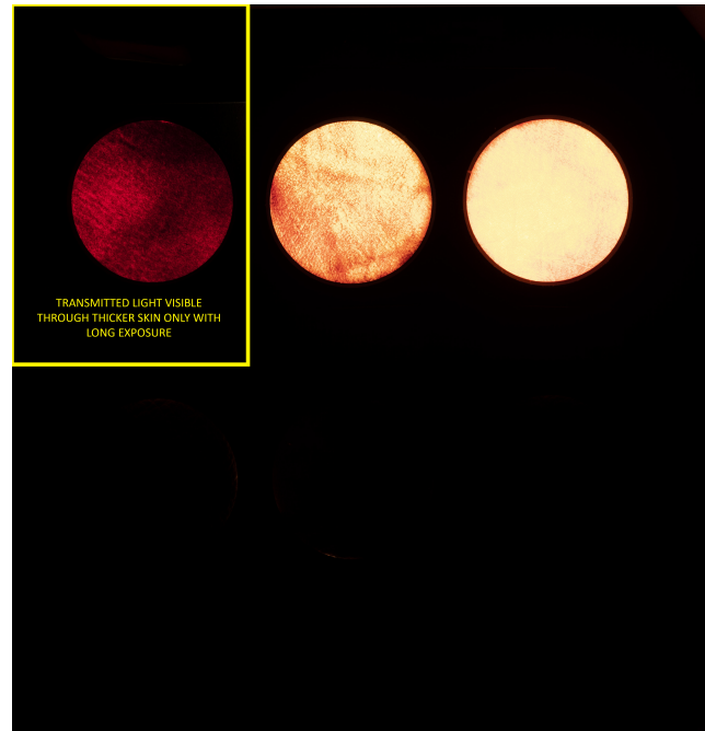
Fig. 3. The same samples as figure 1. Brain-tanned and alum-tawed skins allow transmitted light to pass, while chrome- and vegetable-tanned skins do not.
