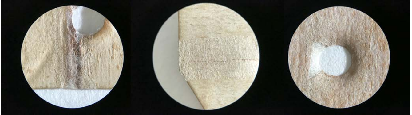
Fig. 14. Photomicrographs (15x magnification) of repairs using 5.0 and 7.3-gram NAJ Tengucho remoistenable tissue ( The Red Man's Greeting (AC85 P7565 893r, Houghton Library, Harvard University).
