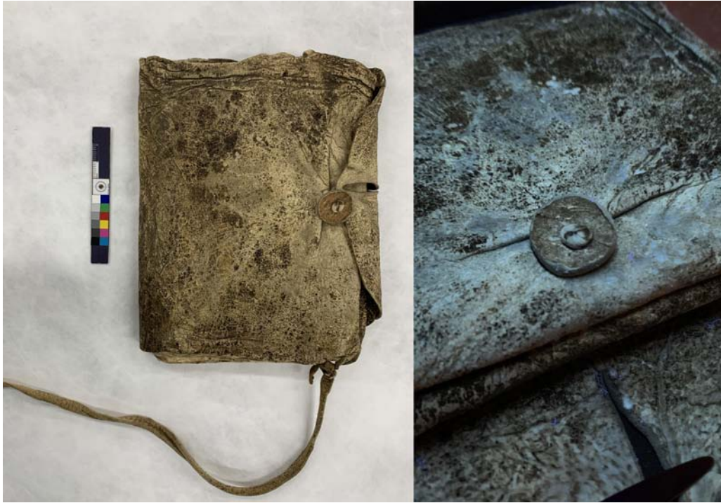
Fig. 5. William Clark, Elkskin Journal, 1805. Courtesy of the Missouri Historical Society, St. Louis. Normal illumination (left) and detail under UV (right). Soft skin wrapper fluoresces and allows transmitted light to pass. In combination with color, tactile qualities, and a well-documented context of production, this evidence strongly indicates that the journal was bound in brain-tanned skin.
