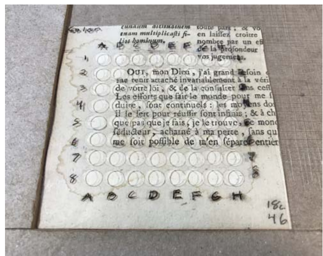
Fig. 4. Polyester film overlay with alphanumeric grid used to avoid the printer’s ink on the antique gelatin paper samples.
