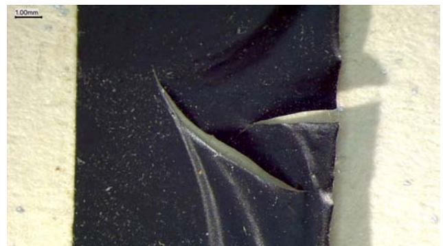
Fig. 7. Micrograph detail of the delamination and the open cracking in the Letraset "r" in one of Schendel's Untitled works (P1970.3.2).
