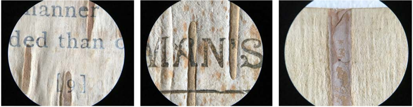
Fig. 3. Photomicrographs (15x magnification) in The Red Man's Greeting (AC85 P7565 893r, Houghton Library, Harvard University); from left to right: betulin, lenticels (inner), lenticel (outer).
