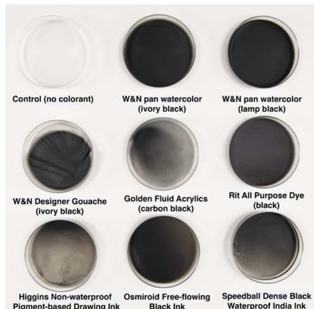
Fig. 8. Dry samples of 0.3% microfibrillated cellulose prepared with the addition of colorants to the slurries prior to casting in a petri dish. Colorants included Winsor & Newton (W&N) watercolors and gouache, Golden Fluid Acrylics, various inks, and dye.
