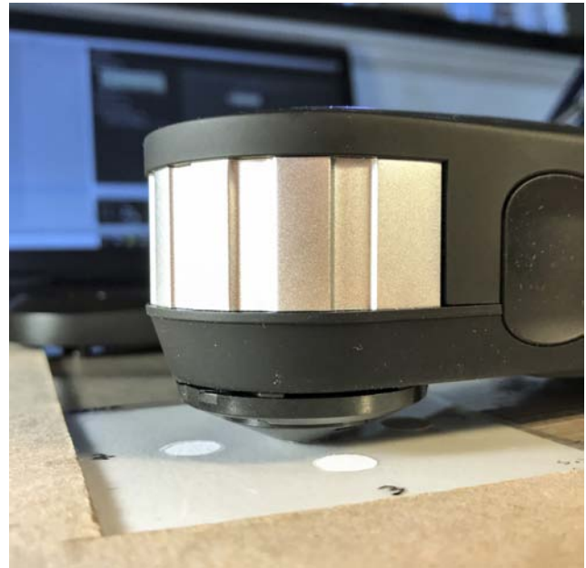
Fig. 3. Spectrophotometer and polyester overlay used to take color measurements of a paper sample.
