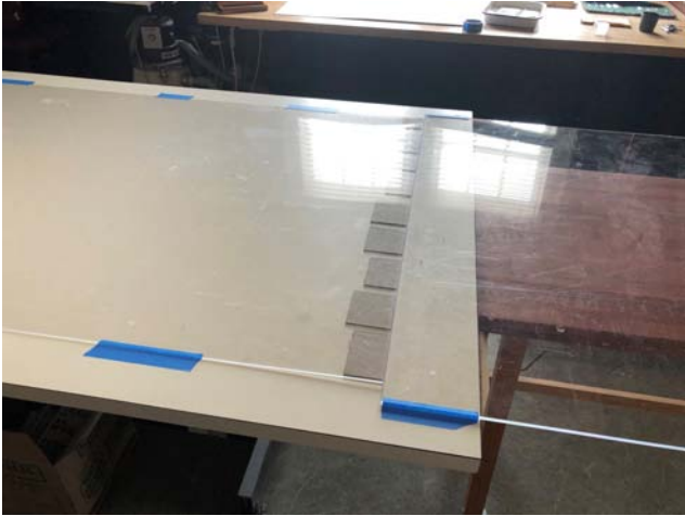
Fig. 9. Acrylic sheets getting shimmed and taped from below create a good seam.
