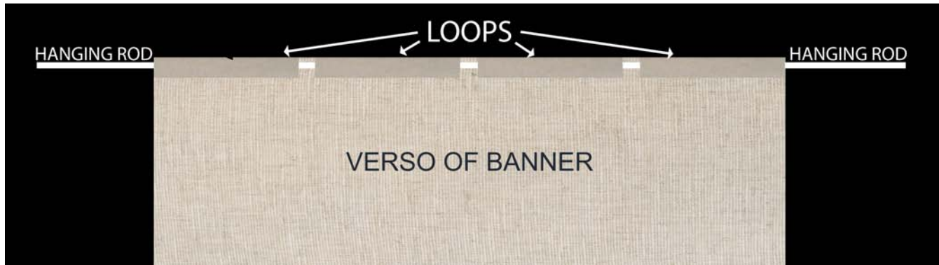
Fig. 13. Diagram of new loop hanging system.
