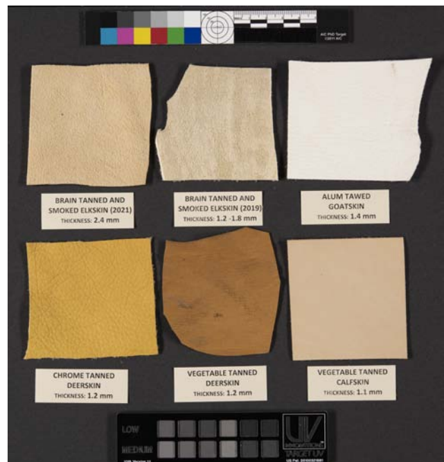
Fig. 1. Samples of brain-tanned, alum-tawed, chrome-tanned, and vegetable-tanned skins under normal illumination. Note the suede surface texture and lack of grain layer in the brain-tanned samples.
