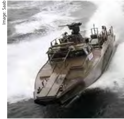
Saab's TRACKFIRE Remote Weapon Station is portrayed here on a CB-90 combat boat from Dockstarvarvet, displaying its ability to remain accurate and independent of boat's movements during High-Speed Boat Operations by using Saab's Fibre Optic Gyros – a vital component in many different platforms.
