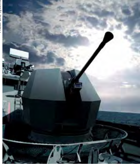
The latest BOFORS 40 Mk 4 version offers full compatibility with the latest 'smart' 3P (Prefragmented, Programmable, Proximity-fused) ammunition.
