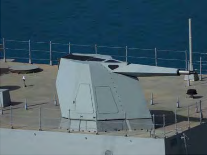
Leonardo has developed a lightweight and non-deck penetrating version of the 76 SR. The 76 Single Deck is installed on the Italian Navy's PPA.
