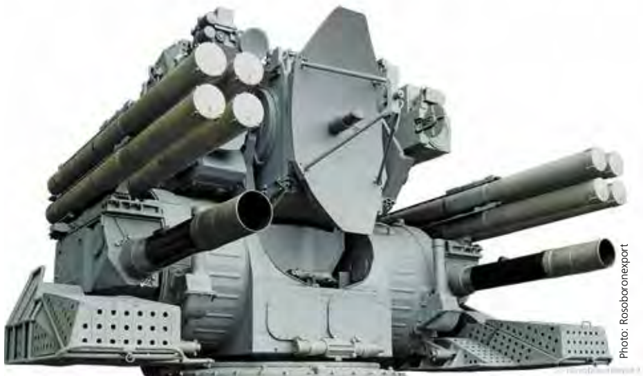
KASHTAN-M is the latest version of this Russian gun/missile system. Improvements include a longer missile and gun ranges, a higher engagement altitude, and a shorter reaction time.
