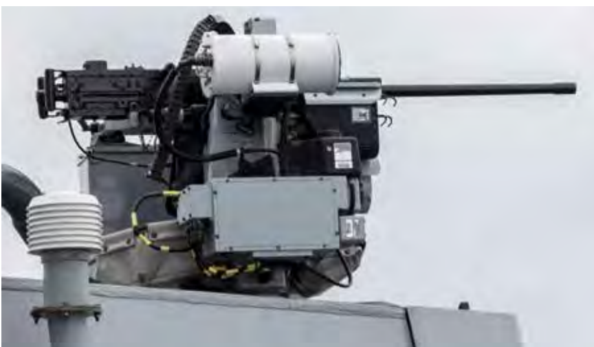
Kongsberg Defence Systems' SEA PROTECTOR Remote Weapon Station for close-in protection at sea is shown here mounted on a Norwegian patrol craft.
