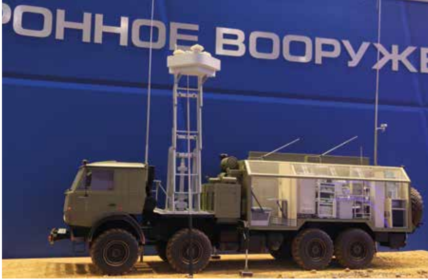
A model of the PREDEL-E mobile over-the-horizon stealth radar
