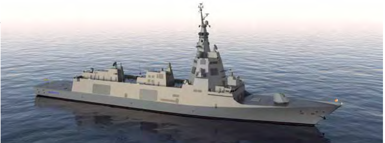
In the scope of the F-110 programme, the Spanish Navy will receive five BONIFAZ class multi-purpose frigates equipped with the AEGIS CWCS. Service introduction is scheduled between 2023 and 2027.
