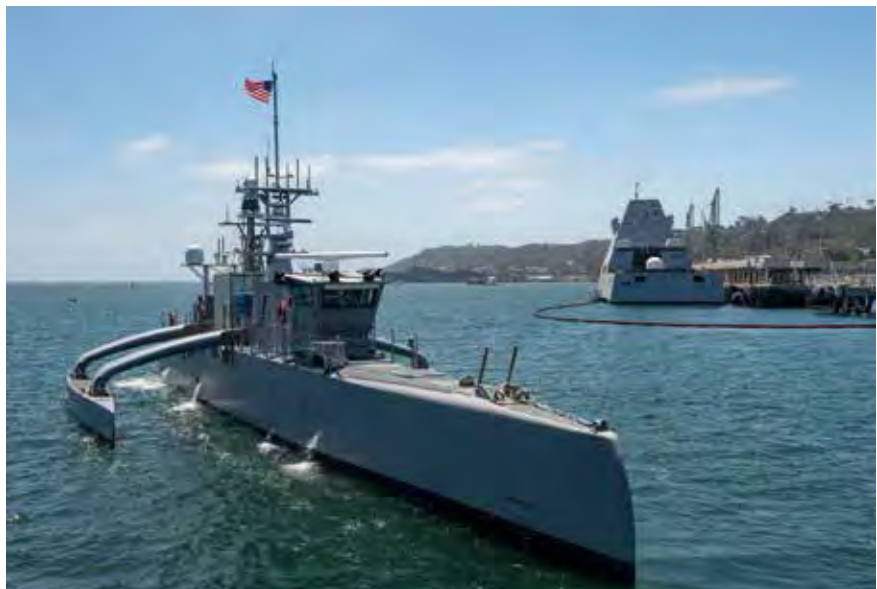
The autonomous USV SEA HUNTER. Large and medium-sized autonomous surface and underwater vehicles will form a steadily increasing part of the US Navy’s fleet.
