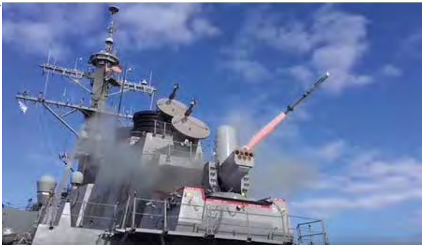
In the SeaRAM system, an 11-cell launcher for the RIM-116A Rolling Airframe Missile (RAM) replaces the 20 mm gun of the PHALANX.
