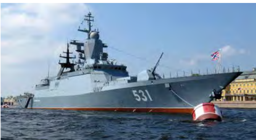
Developed by the JSC Central Research Institute Burevestnik, the 100 mm A-190 gun mount equips mainly frigates and corvettes, like the SOOBRAZITELNY STEREGUSHCHY class Project 20380 corvette.
