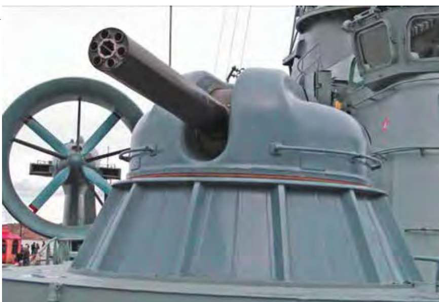
This AK-630M is an improved version of the original AK-630 that was rushed into Soviet Navy service in the early 1970s even before being trials had been completed.
