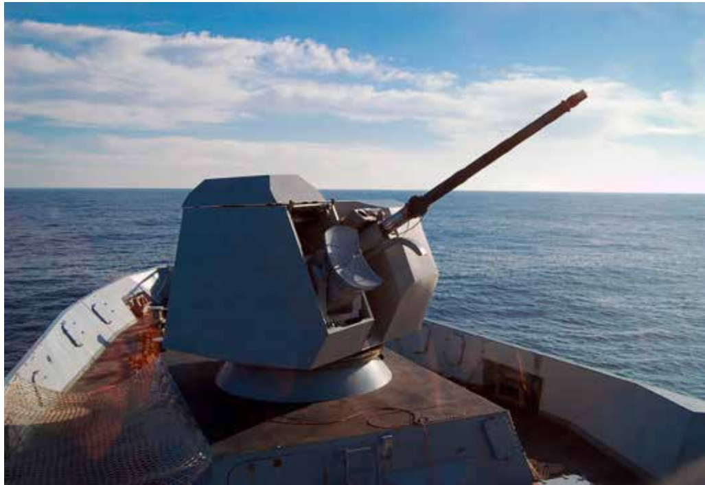
The Leonardo SUPER RAPIDO gun system in the STRALES configuration successfully engaged a subsonic target simulating a sea-skimmer threat.
