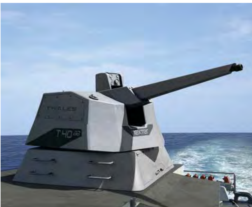
The naval RAPIDFIRE 40 mm gun mount with A3B ammunition will be able to engage aerial threats like drones.
