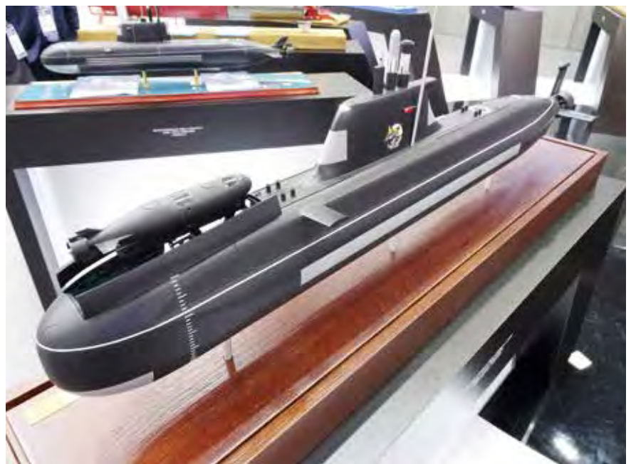
A model of the SERVAL submarine housing a compact TRITON 2 submersible in its bow section.
