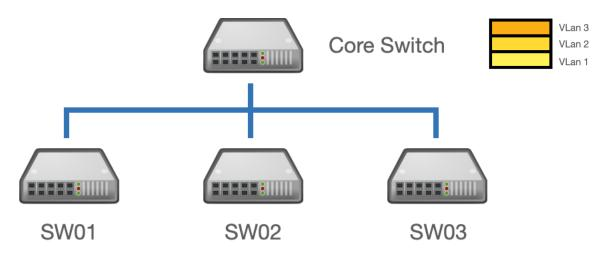
The switches will be broken down into 3 VLANS (Virtual LANs), this is to ensure that traffic is isolated from each other keeping the illusion of 3 separate networks albeit running over the same physical infrastructure.
