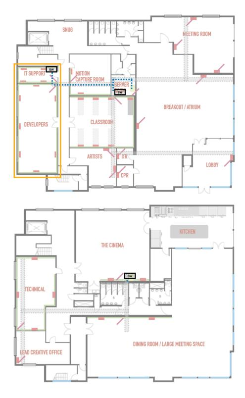
Just the single switch will be installed on the first floor, despite the location being so close to the server room, it was felt that having a single upstairs switch would be a better option. The switch will be connected back via a fibre cable to the core switch in the server room.
