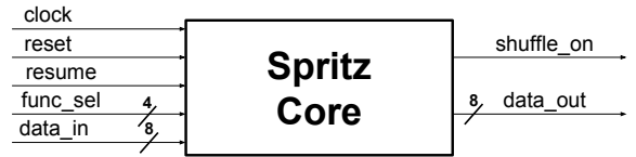
Figure 7: Block diagram of SPRITZ hardware accelerator.
