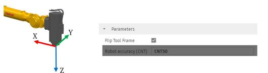
**Note**: if the tool orientation is <u>not</u> one of the above, Autodesk CAM post will not support the application correctly.
