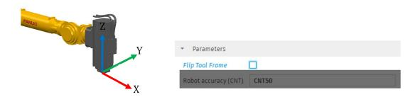
If Z+ is pointing down along the tool axis and X+ is pointing backwards, use Flip option:
