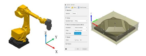
The robot can be jogged along the **User Frame** Coordinate System, this is one option to check the orientation of the **User Frame**.
