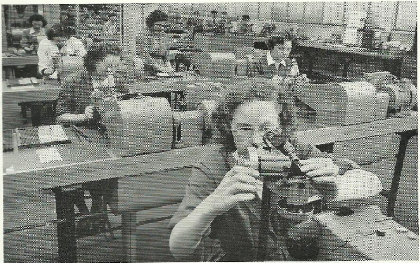
Fig. 17: In the foreground, testing matrices for depth of drive.
