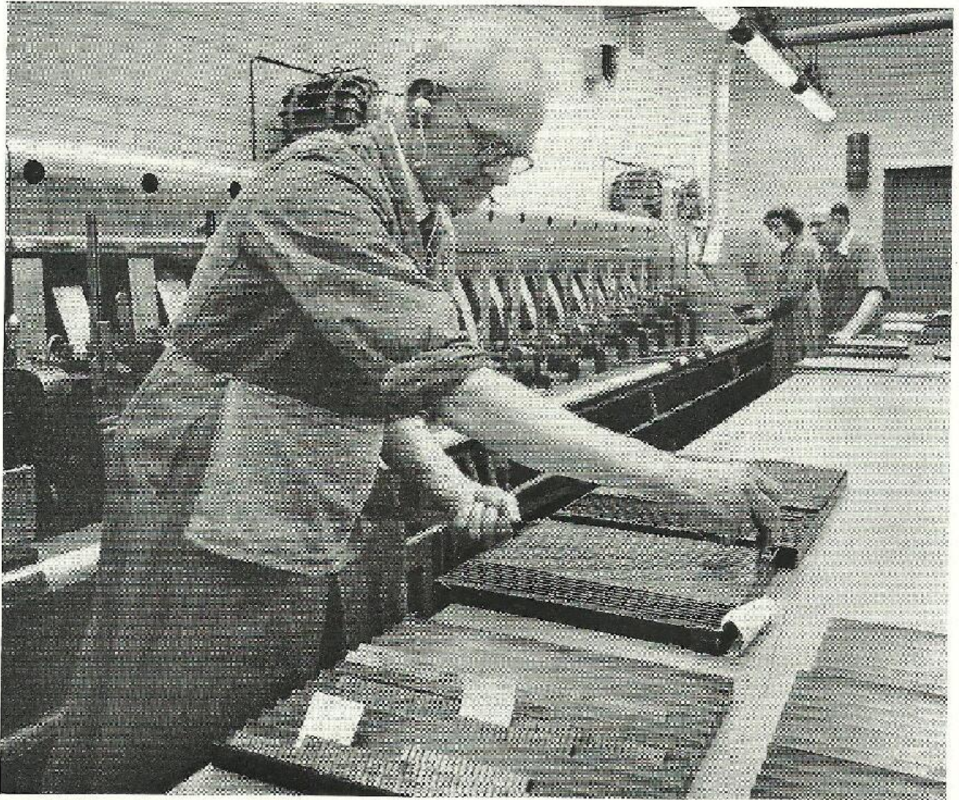
Fig. 19: A galley of composition matrices about to be lapped to size.
