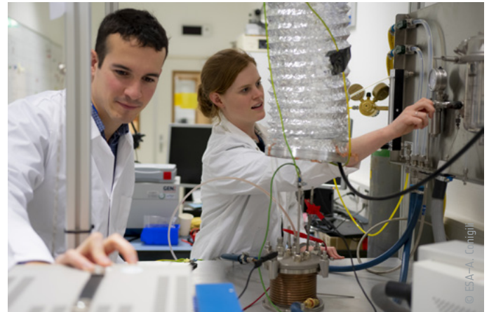
▲ Producing oxygen and metal out of simulated moon dust inside ESA's Materials and Electrical Components Laboratory
