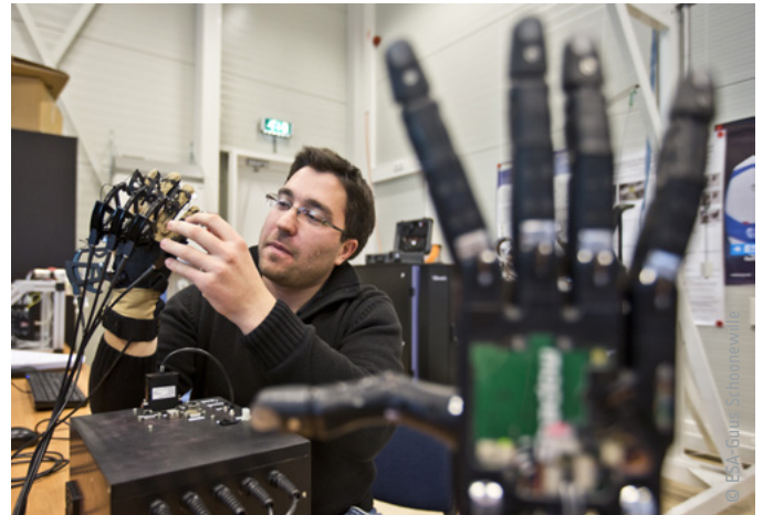
▲ When the ESA engineer moves his gauntleted hand, the robotic hand follows in sync
