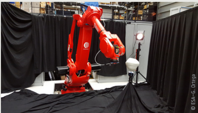
▲ Preparing the practical test of the navigation of Hera around Didymos
