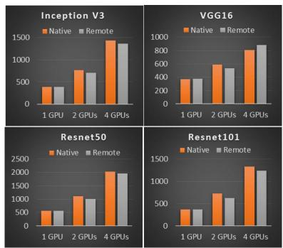
Figure 3: Performance comparison of Network Attached Remote GPUs with FlexDirect on Dell EMC PowerEdge Servers vs. Native GPU execution Performance is represented on y-axis (images/sec, higher is better), for training different CNN models using Tensorflow.
