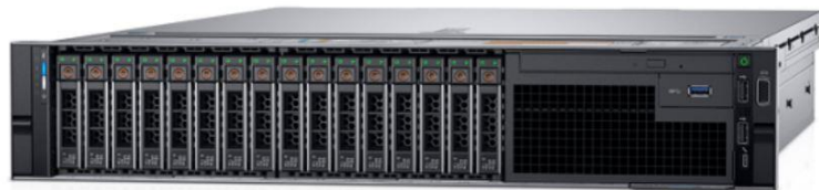
Image 1: The 2-socket, 2u, PowerEdge R740 rack server
