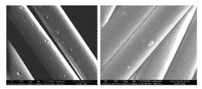
Figure 6. a SEM of polyester yarn with 110ppm H<sub>3</sub>PO<sub>4</sub> Figure. 6 b SEM of polyester yarn 125 ppm H<sub>3</sub>PO<sub>4</sub>
