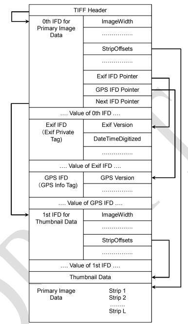
Figure 6 Basic Structure of Uncompressed Data Files
