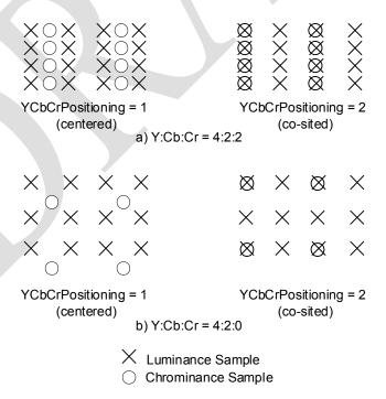
Figure 13 YcbCrPositioning
