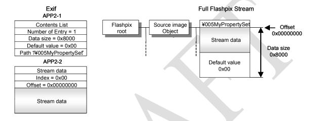
Figure 61 Conversion to Flashpix Extensions (1)
