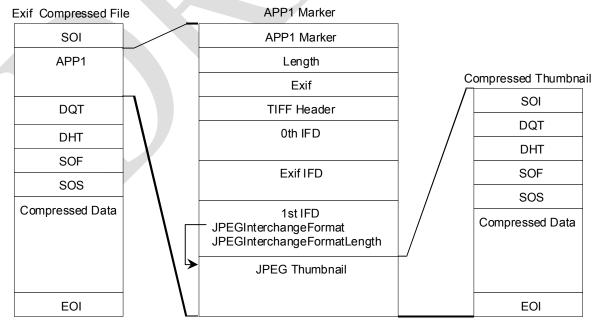
Figure 9 Structure of Exif file with compressed thumbnail
