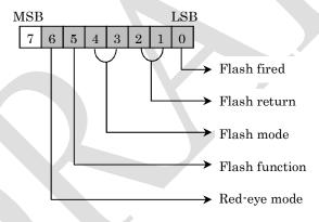
Figure 16 Bit Coding of the Flash Tag
