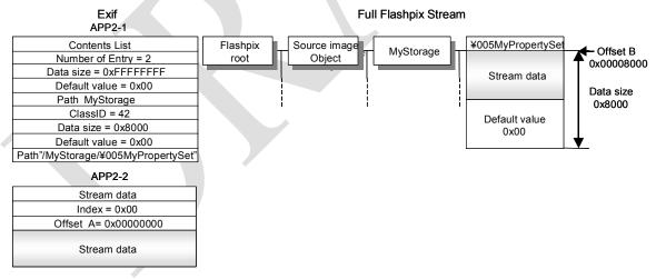
Figure 63 Conversion to Flashpix Extensions (3)
