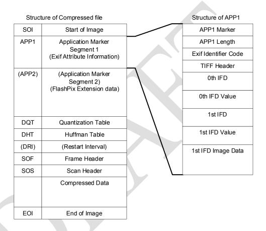
Figure 7 Basic Structure of Compressed Data Files
