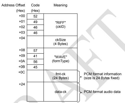
Figure 44 Basic Structure of PCM Format
