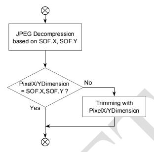
Figure 37 Procedure for Image Data Reproduction
