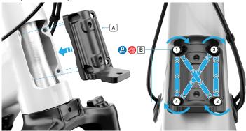
■ Insert the bolts (B) through the head plate (A) into the head tube mounting holes, then using a 4mm hex bit and torque wrench, torque the bolts to 4.5 Nm / 40 in-lbf.
