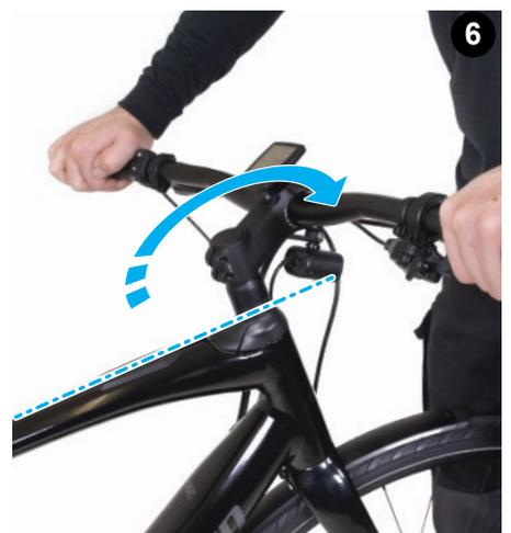
7. Align the handlebar with the center of the bicycle.
