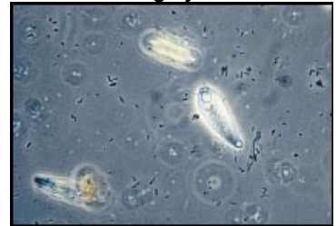
4b A variety of rod-shaped bacteria and two protozoans found in a recirculating cooling system.
