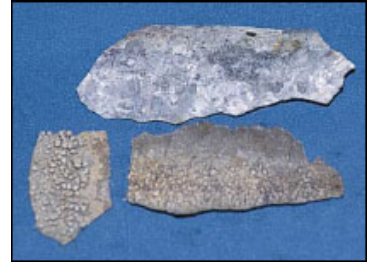
2b. Curved scale chips that broke away from a large diameter pipe.
