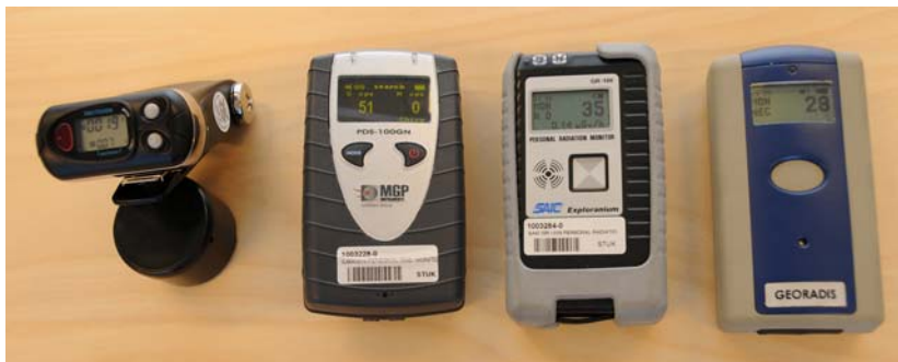
Figure A8.3. Examples of Personal Radiation Detectors (PRDs). All except one (second from right) are also spectrometers. All except one (right) include neutron monitoring option. Photo: STUK.
