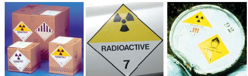
Figure E3. Packages and vehicle with potentially dangerous sources symbol. Photos: HPA
