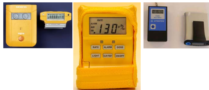
Figure A8.2. Examples of personal alarming dosimeters. Photos: HPA, STUK.
