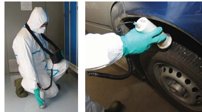
Figure F9. Alpha contamination monitoring. This photograph illustrates the method, but when responding to an incident, additional measures would need to be employed, i.e. the detector would be wrapped in plastic film with the exception of the front window. Photos: STUK.
