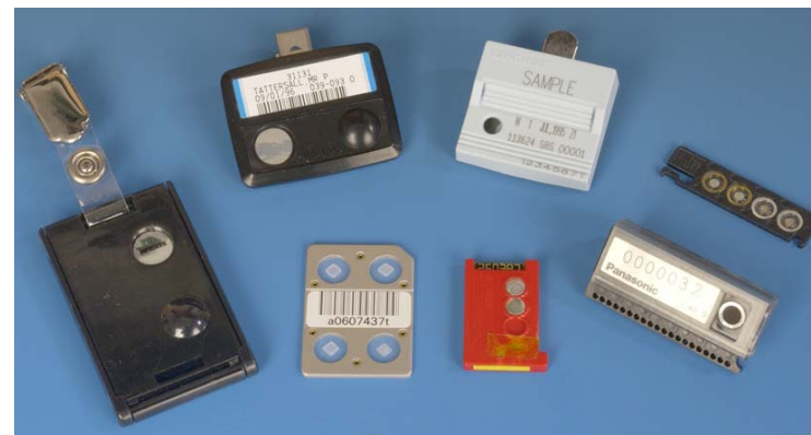
Figure A8.4. Examples of ThermoLuminescent Dosimeters (TLDs). Photo: HPA.
