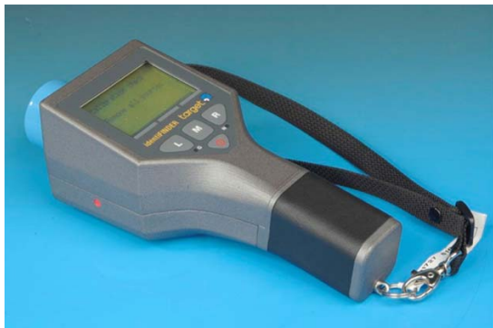
Figure A8.11. Example of portable gamma spectrometry equipment. Photo: STUK.
