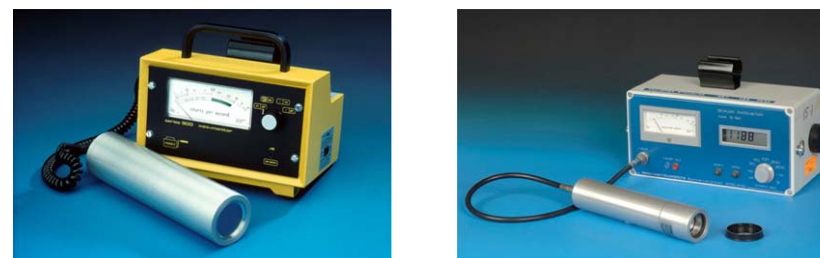
Figure A8.10. Examples of NaI(Tl) detector based monitors used as gamma contamination monitors. Photos: HPA.
