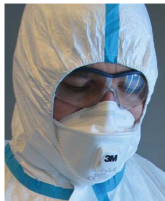
Figure A2.3. Filtering facepieces (FFP) are classified into three classes FFP1, FFP2 and FFP3 with filter material penetration factors less than 20 %, 6 % and 1 %, respectively. Extra inward leakage from the edges lead to total allowed inward leakages less than 22 %, 8 % and 2 %. Only FFP3 filtering facepieces give a good protection factor (NPF 50) for prolonged exposures. They are adequate for personnel working outside the Red Zone. Photo: STUK.
