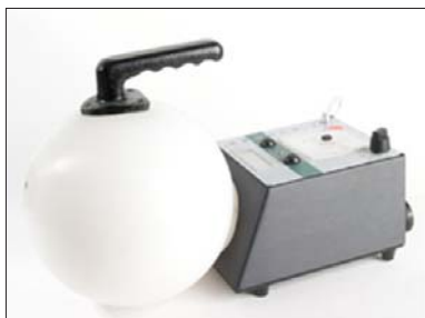
Figure A8.9. Example of a hand held monitor for measuring neutron dose rate. Photo: HPA.
