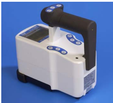
Figure A8.5. An example of a beta dose rate monitor. Photo: HPA.
