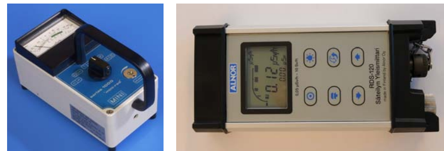
Figure A8.1. Examples of gamma dose rate monitors. Photos: HPA (left), STUK (right).
