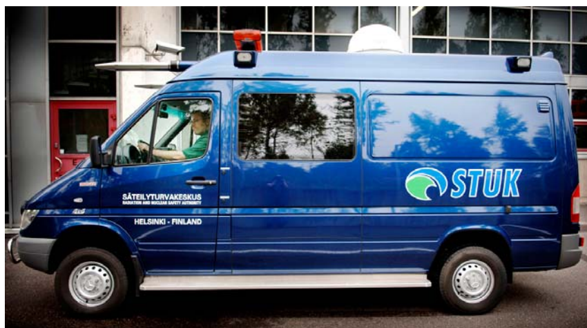
Figure A8.13. An example of a radiation surveillance vehicle and mobile laboratory. The laboratory is equipped for dose rate monitoring, nuclide identification, aerosol sampling, sample and in situ gamma spectroscopy measurements and alpha spectroscopy measurements, as well as operational voice and data communication. Photo: STUK.
