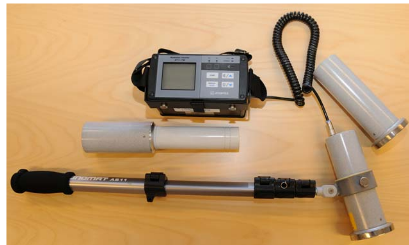
Figure A8.8. An example of alpha, beta and gamma contamination monitor. Photo: STUK.
