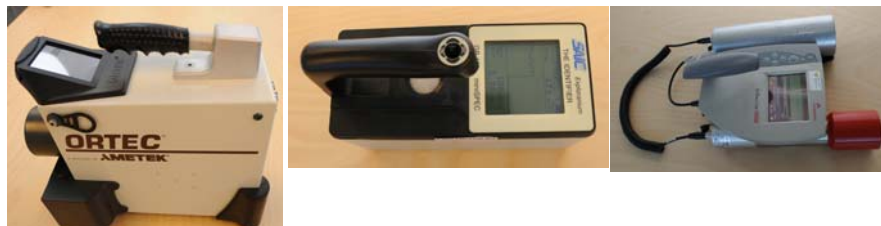
Figure A8.12. Examples of Radionuclide Identification Devices. All are gamma spectrometers with a neutron monitoring option. Photos: STUK.
