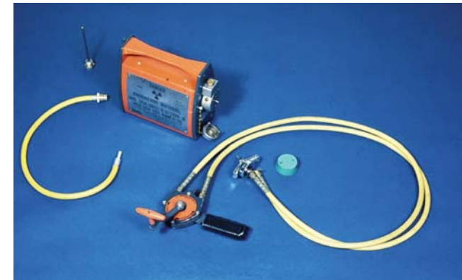
Figure E4. Typical radiography camera. Photo: HPA.
