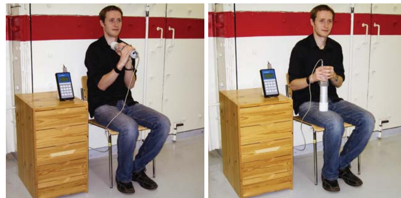
Figure F14a. Measurement of ^{131}\text{I} in the thyroid.
