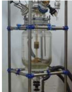
Supplementary Figure 1 | Picture of reactor (20 L) for the scalable preparation of GO Fe .
