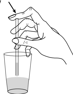
Figure 4.11. Gravity pulls the water down, increasing the volume and lowering the pressure of the trapped air.
