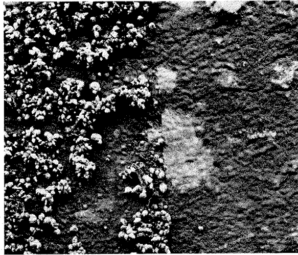
FIGURE 2. Comparison of fouling on old Navy formulation 15RC (left), and modern hot plastic antifouling paint (right), after 17 months waterborne. Official U. S. Navy photograph.
