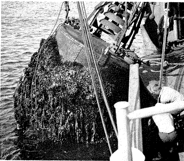
FIGURE 6. Navigation buoy heavily fouled with mussels and Laminaria .
