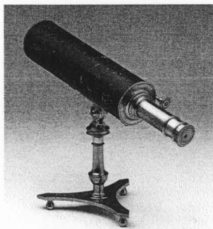
180. 8162 Gregorian reflecting telescope on tripod stand 1750-1800 h 18, w 26, d 10.5 Provenance: J. van Bennekom, 1930
