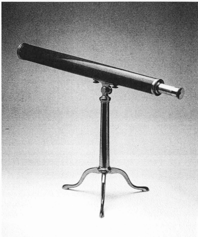
115. 11915 & 15005 Refractor on small tripod c. 1775 l 73.5-118, Ø 6.0-7.0 Signed on the end of the tube: DOLLOND LONDON. Provenance: J.H.C. Lisman, Leiden, 1931
