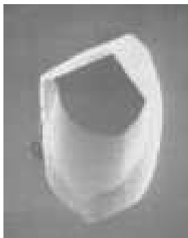
Figure 6-2: An SEM micrograph of a calcite crystal grown in 0.01M L-Asp by Orme et al. The rounded acute steps and the sharp obtuse steps can clearly be seen on the crystal.
