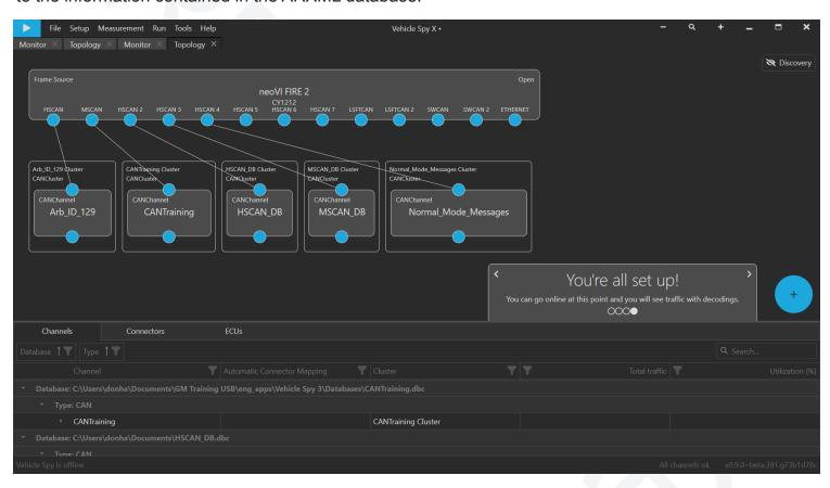
AUTOSAR ARXML file loaded and ready for Restbussimulation. All ECUs are simulated., traffic using a bus capture (Simulation VSB) as the Frame Source.
