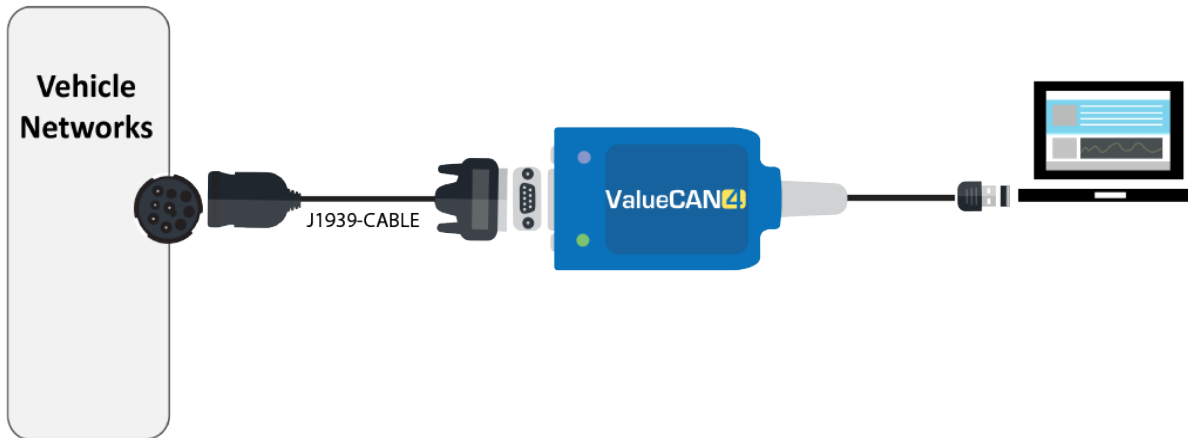
Figure 7: Connector Diagram with ValueCAN Deutsch 9-Pin (J1939-RP1210) Cable (DB-9F to Deutsch 9-Pin) Part # J1939-CABLE
