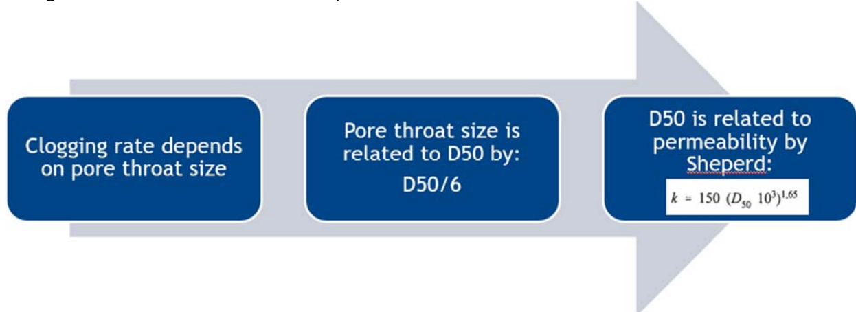
Figure 10 Workflow for relating permeability to pore throat size
