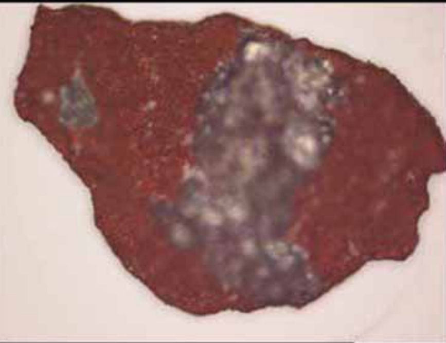
Partially reacted thermite chips
