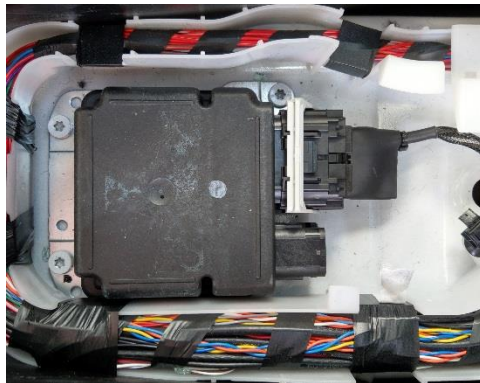
Figure 45. Connecting the EDR Retrieval Cable to the RCM 2/4
