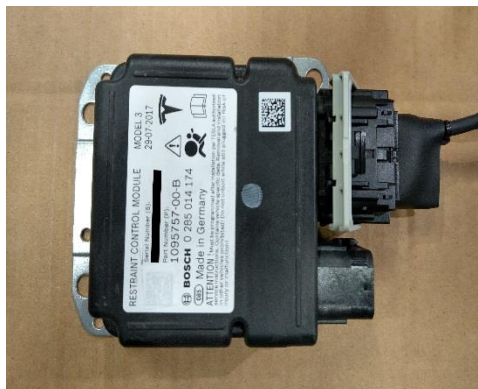
Figure 58. Connecting the EDR Retrieval Cable to the RCM 2/4
