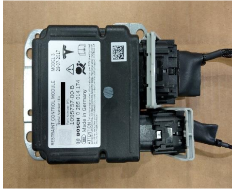
Figure 59. Connecting the EDR Retrieval Cable to the RCM 3/4
