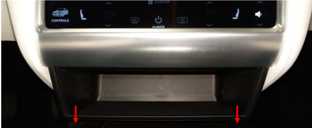
Figure 2. Releasing the storage pocket
