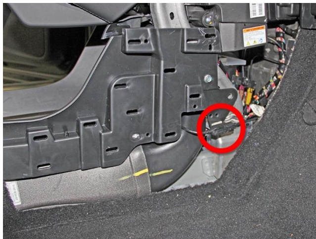
Figure 32. Disconnecting the center console front USB electrical connector
