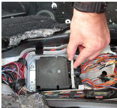
Figure 41. Disconnect the RCM connectors 1/3
