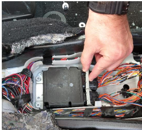
Figure 52. Disconnect the RCM connectors 1/3
