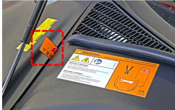
Figure 68. Opening the first responder access panel
