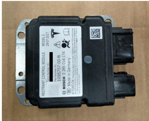
Figure 56. RCM removed from the vehicle
