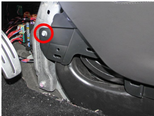
Figure 30. Bolt securing the front LH side of the center console
