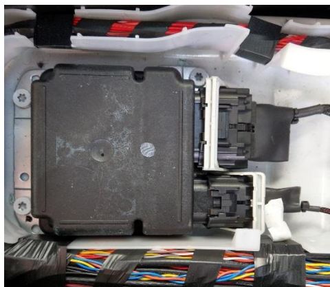
Figure 46. Connecting the EDR Retrieval Cable to the RCM 3/4
