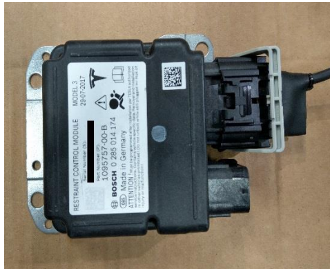
Figure 57. Connecting the EDR Retrieval Cable to the RCM 1/4
