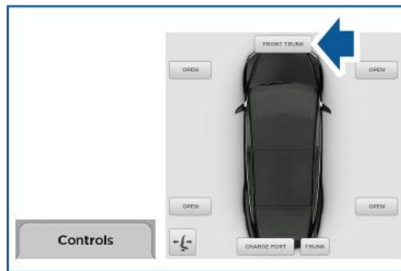
Figure 64. Opening the front trunk using the touchscreen
