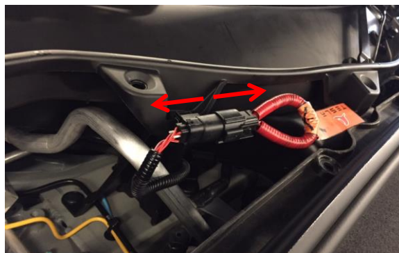
Figure 70. Disconnecting the first responder loop harness
