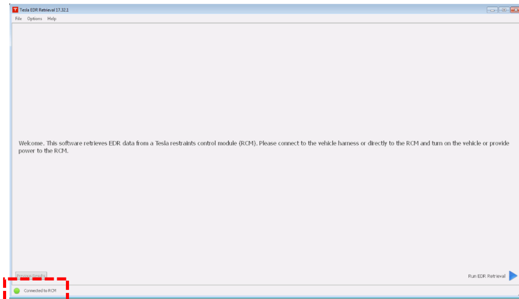
Figure 72. EDR program successful connection
