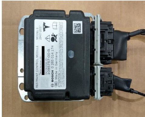
Figure 60. Connecting the EDR Retrieval Cable to the RCM 4/4
