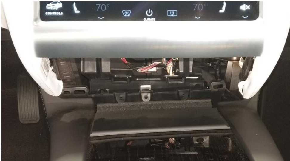
Figure 3. Removing the storage pocket
