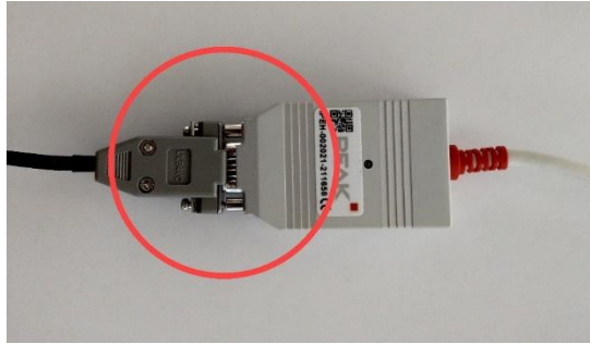
Figure 45. Connecting the EDR retrieval cable to the PCAN
