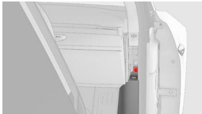
Figure 3. Releasing the A-Pillar Lower trim
