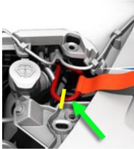
Figure 50. Front First Responder Loop
