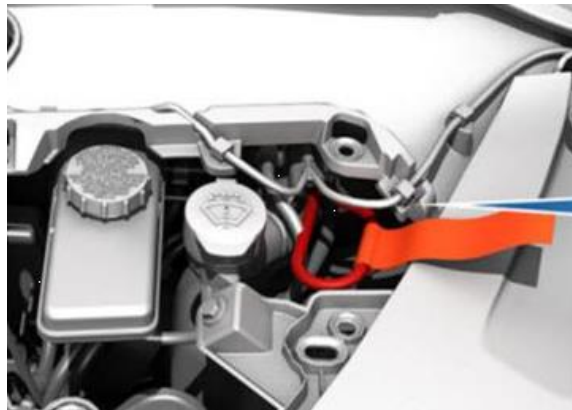
Figure 11. Front First Responder Loop
