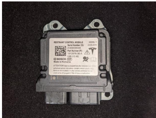
Figure 44. RCM removed from the vehicle and ready for connection
