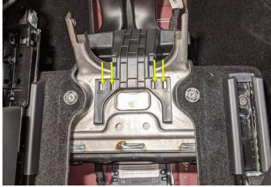
Figure 40. Center console support bracket tabs
