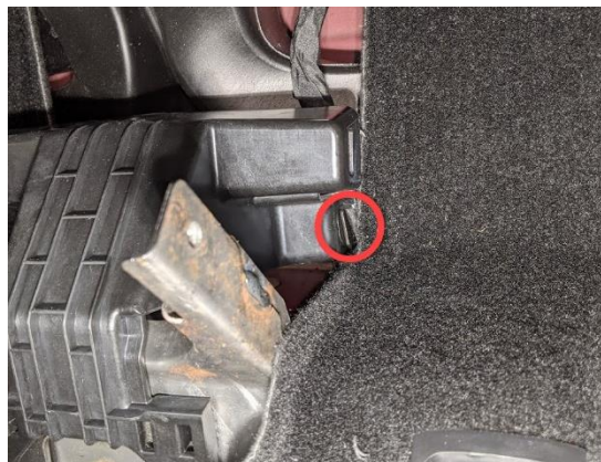
Figure 39. Center console support bracket clip
