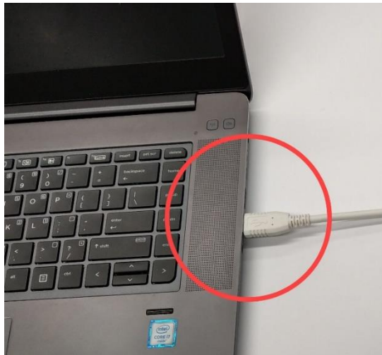
Figure 20. Connecting the PCAN to the computer
