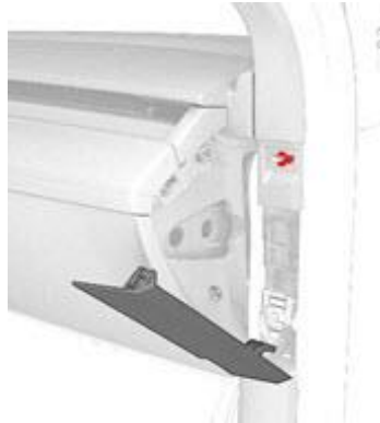
Figure 2. Removing the A-Pillar Middle trim
