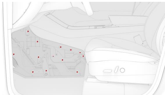
Figure 22. Center console side panel clip locations
