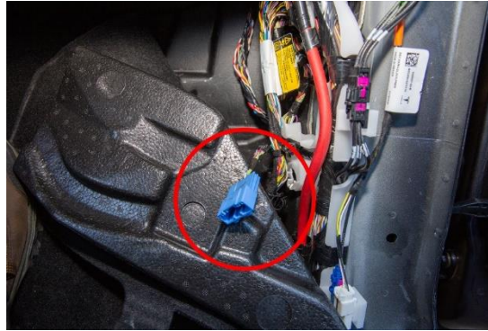
Figure 7. The CAN bus connector in position
