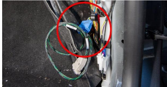
Figure 8. The In-Vehicle EDR Retrieval Cable connected to the CAN bus connector
