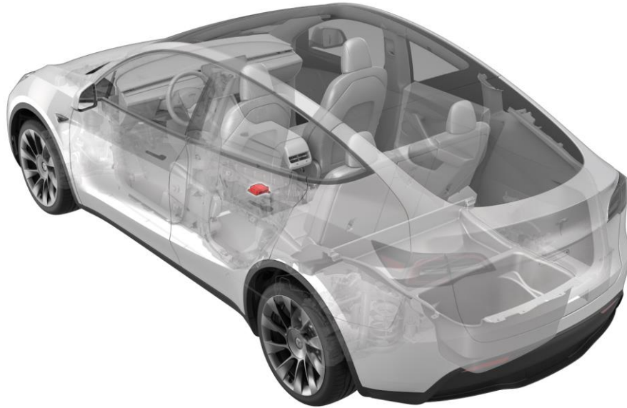
Figure 21. Model Y RCM location
