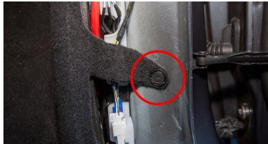
Figure 5. Detaching the RH passenger side carpet
