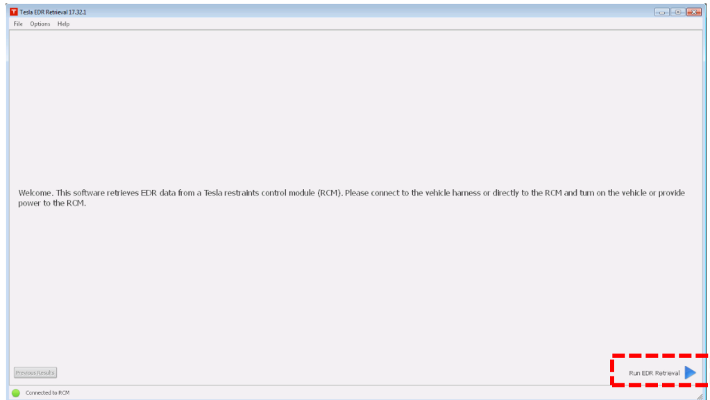
Figure 51. Retrieving data using the Tesla EDR retrieval program
