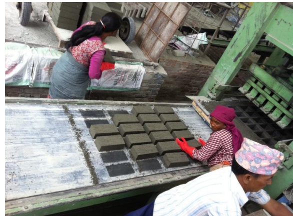
Figure 2.1 Production of compressed bricks in Nepal
