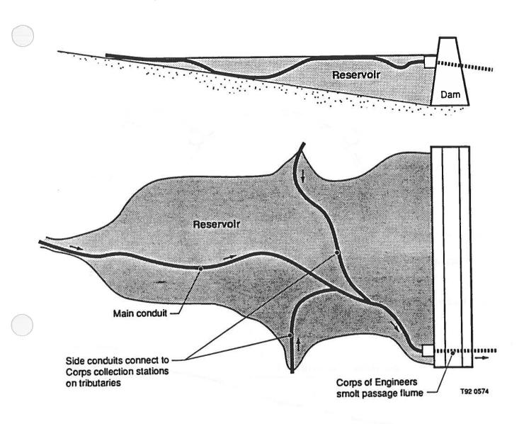
Figure 1. This conduit system has both surface and submerged sections and can be configured to reach all the tributaries draining into a reservoir if necessary.
