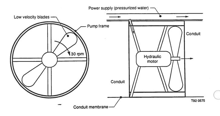
Figure 5. The pumping section of the conduit is a separate unit used to connect the individual membrane sections together. The unit is designed to operate on the surface or in the submerged sections, deriving its power from the pressured water line which runs the length of the conduit.
