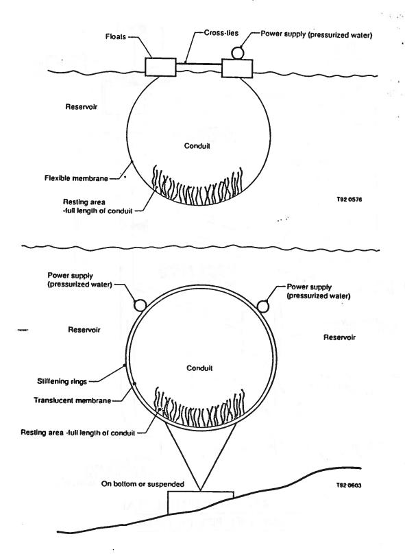
**OPEN CHANNEL AND CLOSED CONDUITS - TYPICAL INEL PIPELINE SECTIONS**
