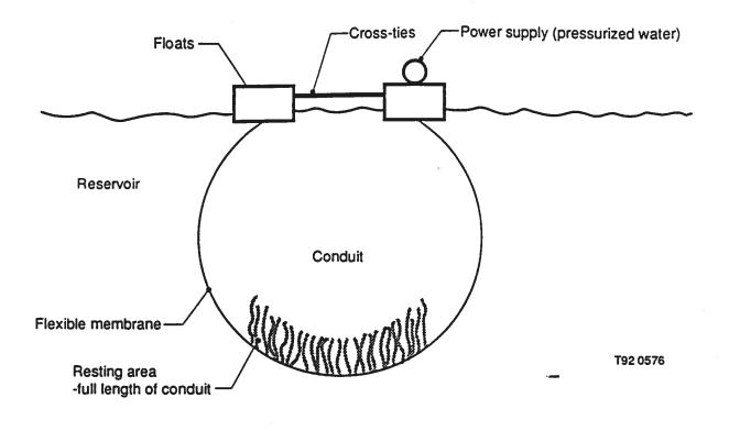
Figure 3. The conduit is a very light, flexible membrane which is supported in the reservoir by floats, which are held together by a series of crossties. The power supply carries high-pressure water for the pumping sections. A resting area in the bottom of the conduit will be provided the entire length of the conduit.
