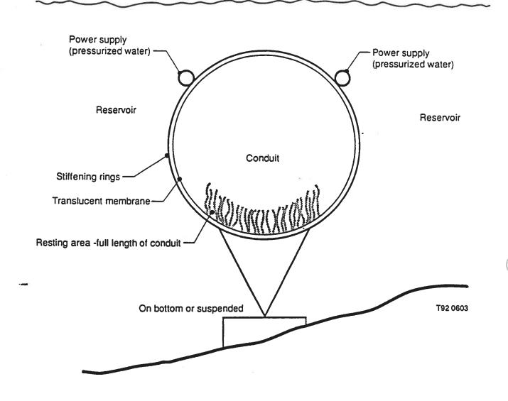
Figure 2. The conduit is completely closed in the underwater sections to avoid the fish escaping into the reservoir water. The conduit is anchored to the bottom. Since the design is only conceptual at this point, the figure is meant to be illustrative only. Final design will dictate the size of anchors, restraining cords, attachment process, and flotation devices.
