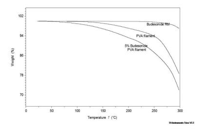
**Figure 4.** TGA thermal traces for budesonide (raw material), PVA and budesonide-loaded PVA filaments.
