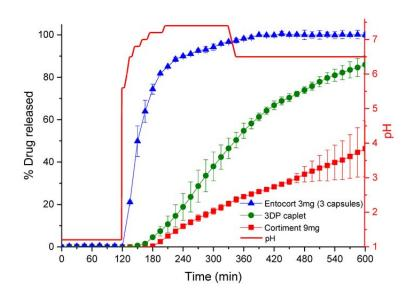
**Figure 7.** Drug release from Cortiment<sup>®</sup>, Entocort<sup>®</sup> and coated 3D printed caplets in 0.1M HCl for 2h followed by physiological bicarbonate buffer under dynamic pH conditions (pH 5.6 to 7.4 and then 6.5) controlled by the Auto pH System<sup>TM</sup>. Red line shows the real-time pH values.
