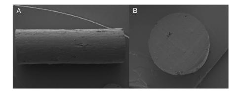
**Figure 3.** SEM images of (A) surface view and (B) cross section of budesonide loaded PVA filament after HME.
