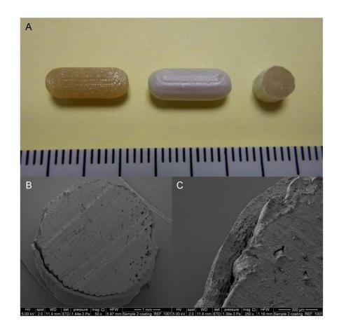
**Figure 6.** Images of 3DP fabricated caplets (A) from left to right, caplet prior to coating, caplet after coating and cross section of coated caplet (scale in cm); (B,C) SEM images of internal structure of cross-section of a coated-3D printed caplet.
