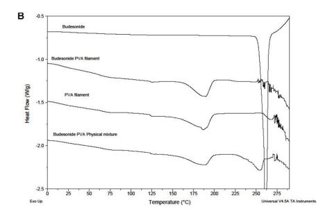
**Figure 5.** (A) X-ray powder diffractograms of pure budesonide and 3D printed discs of PVA and budesonide-PVA (B) DSC thermograms for Budesonide, PVA, budesonide-loaded PVA filaments and a physical mixture of PVA and the drug.
