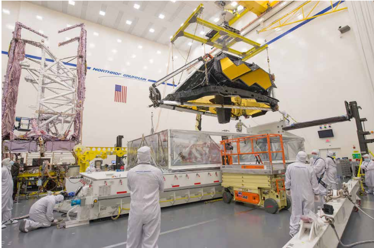
Figure 2. James Webb Space Telescope elements in the clean room at Northrup Grumman Space Park, including the spacecraft element (far left) and payload element (top center).
