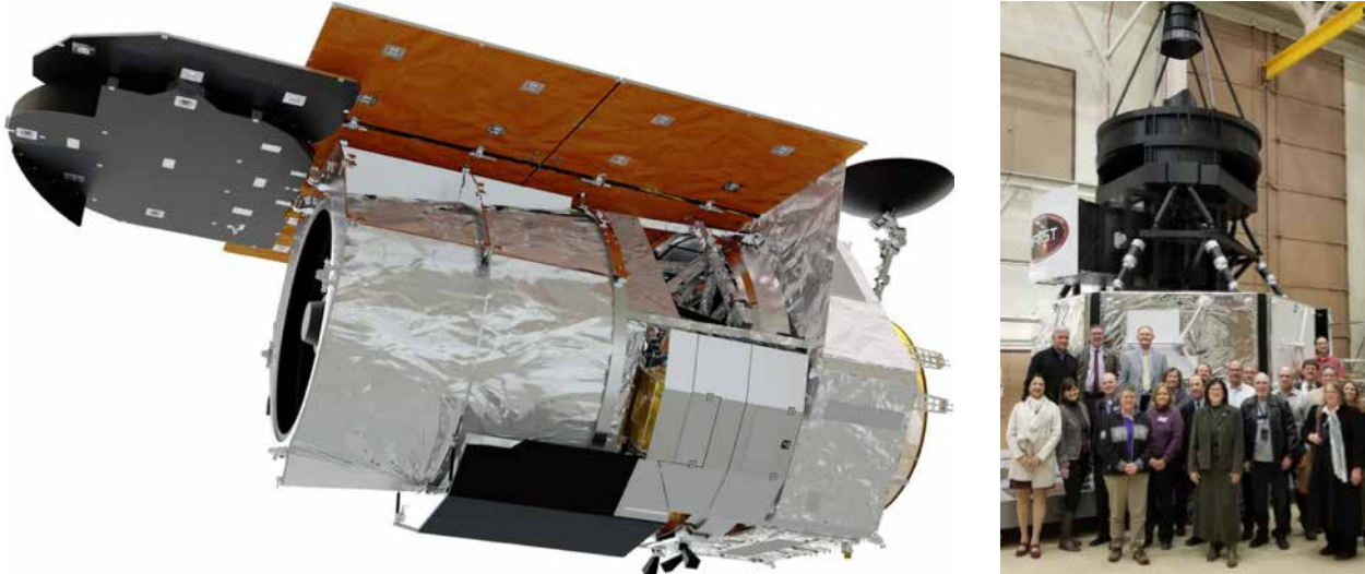
Figure 4. Mid-2018 design of WFIRST (left) and a full-size mockup without the outer barrel assembly (right), illustrating the scale of the observatory.
