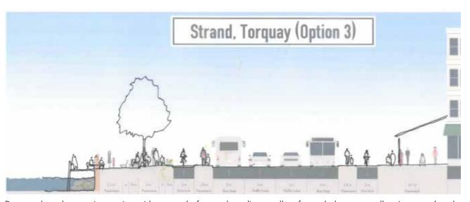
Proposed road narrowing option with removal of central median to allow for cycle lanes as well as increased pedestrian zones. This option would need to be considered against a wider cycle network strategy for the town centre and harbour.
