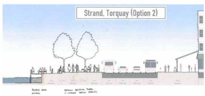
Proposed road narrowing option with removal of central median to widen the footway zones. Multiple crossings provided. Potential for additional public 'deck' zone over the harbour edge in accordance with the harbour plan.
