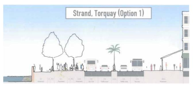
Proposed road narrowing option with retention of central median but as a crossing point rather than a barrier.
