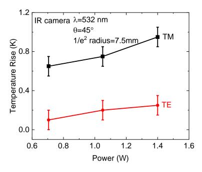
Fig. S2. Water surface temperature rise as a function of laser power. The radius of air-water interface is 15 mm. Incident laser power is 1.4 W.
