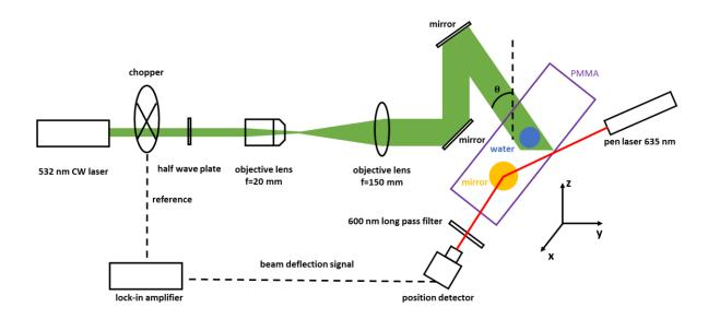
Fig. S23. Optical path of modulated cantilever beam measurement. The glass container of the water is not displayed in the figure.
