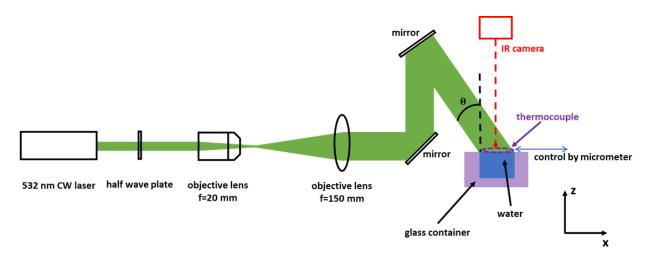
Fig. S1. Optical path for water surface temperature measurement.
