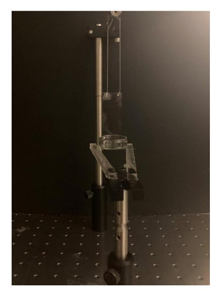
Fig. S31. Set-up of vertical vapor phase temperature distribution.
