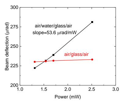
**Fig. S9. Beam deflection signal of SS-TBD as a function of power.** The wavelength of the laser is 635 nm. The polarization of the laser is TM. Black squares represent air-water/glass/air sample. Red circles represent air/glass/air sample.
