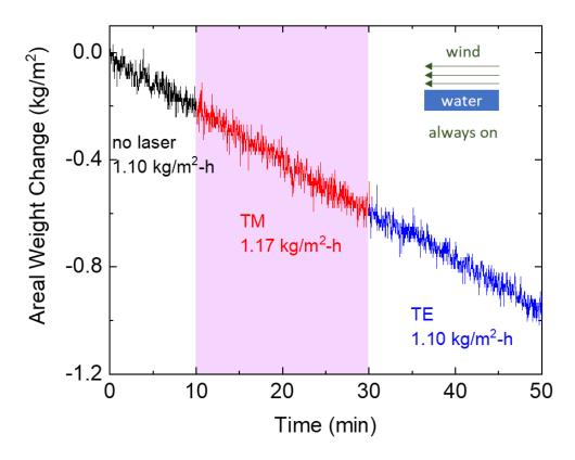
Fig. S28. Areal weight changes as a function of water under air flow. The power of laser is 1.0 W and the radius of air-water interface is 15 mm. Power/areal of water surface  $\approx 1400 \text{ W/m}^2$  (1.4 suns).
