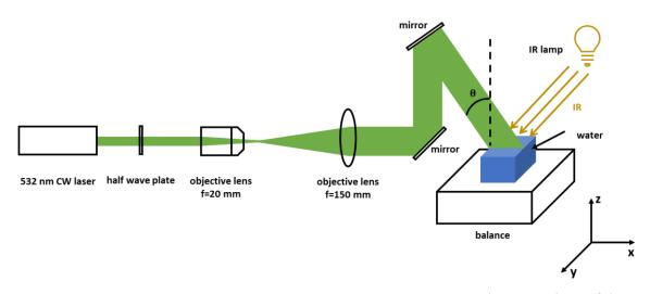
Fig. S26. Optical path of evaporation measurement with IR lamp. Glass container of the water is not displayed in the figure.
