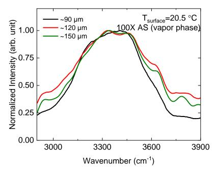
Fig. S20. Evolution of Raman spectra. The working distance of 100X lens is 0.21 mm. The  $1/e^2$  radius of green laser (532 nm) at beam waist is ~0.5  $\mu$ m. The average distance of beam waist above air-water interface is ~90  $\mu$ m (black line), 120  $\mu$ m (red line), and 150  $\mu$ m (green line) during each measurement.
