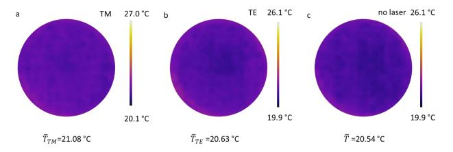
**Fig. S25. IR image the absorption estimation measurement**. (a) IR image under TM-polarized illumination (wavelength 532 nm, power 1.4 W, incident angle 45°, 1/e<sup>2</sup> radius 3.75 mm) (b) IR image under TE-polarized illumination. (c) IR image without laser.
