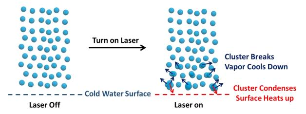
Fig. S5. Schematic of temperature response in the vapor phase and on liquid surface due to the photomolecular effect. Some clusters condense onto the water surface, heating up water. Some clusters break up in air, cooling down air.
