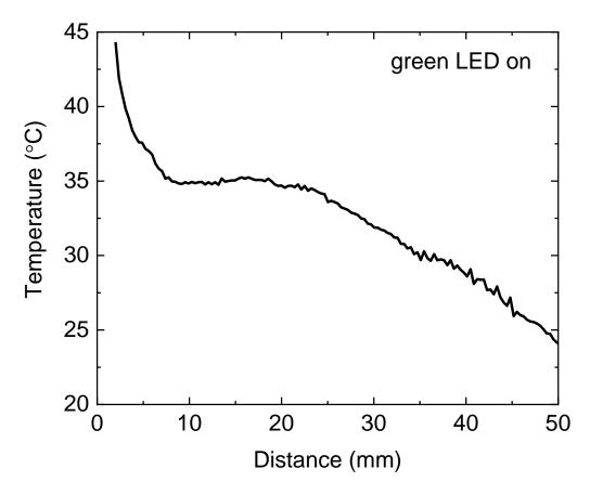
Fig. S17. Vapor phase temperature distribution under LED illumination. The wavelength of LED is 520 nm. The incident angle is  $30^{\circ}$ . The surface temperature is  $\sim 55^{\circ}$ C before LED on. The intensity of green LED is  $1000 \text{ W/m}^2$ .
