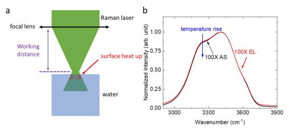
Fig. S33. Raman thermometer measurement. (a) Schematic of water surface heat up by photomolecular effect under Raman laser illumination; (b) Raman spectrum above water surface (100X EL and 100X AS). Working distance of 100X lens is 0.21 mm. The  $1/e^2$  radius of green laser (532 nm) at beam waist is ~0.5  $\mu$ m. Surface temperature of water is ~20.5 °C before laser turns on. The power of laser is 17 mW. Black curve is measured with the average distance of beam waist over water ~30  $\mu$ m.
