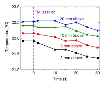
Fig. S4. Temperature response of vapor phase temperature at different height above airwater interface. Time zero is defined when the laser turns on. The incident angle of light is 45°.
