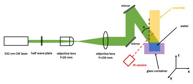
Fig. S3. Optical path of vapor phase temperature distribution image above water surface.
