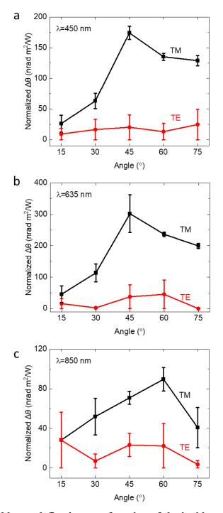
Fig. S13. Normalized beam deflection as a function of the incident angle.
