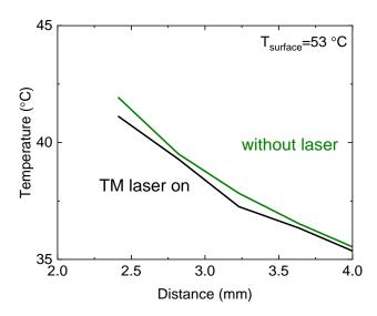
**Fig. S16. Vapor phase temperature distribution above hot water.** Black solid line represents steady-state vapor temperature profile with TM-polarized light (wavelength 532 nm, power 1.4 W, incident angle 45°, 1/e² radius 7.5 mm). Green solid line represents steady-state vapor temperature profile without laser. The radius of air-water interface is 15 mm. Surface temperature of water is 53 °C before laser turns on. The polarization of the laser is TM.
