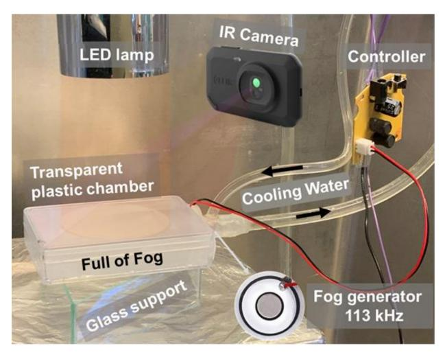
**Fig. S29. Fog experimental setup.** Fog generated by an ultrasonic vibrator is injected into a plastic container. The ultrasonic vibrator is cooled to avoid heating the fog.
