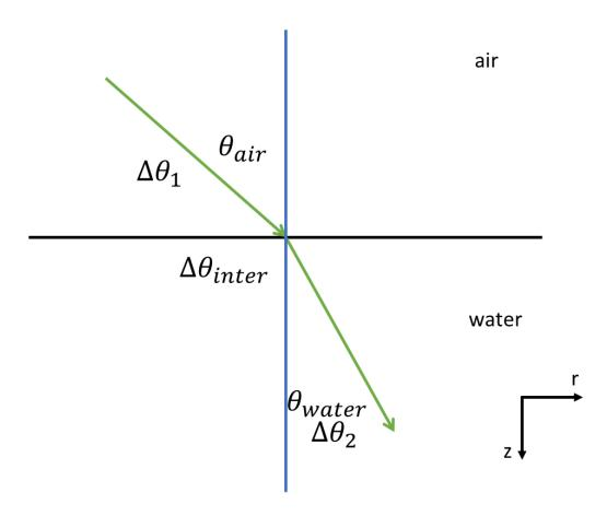
Fig. S10. Display of beam deflections from temperature field at air-water interface.  $\Delta\theta_1$ ,  $\Delta\theta_{inter}$ , and  $\Delta\theta_2$  are the beam deflection in the air phase, air-water interface and water phase respectively.
