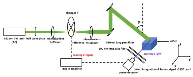
Fig. S21. Optical path for  $2\omega$  Raman measurement.
