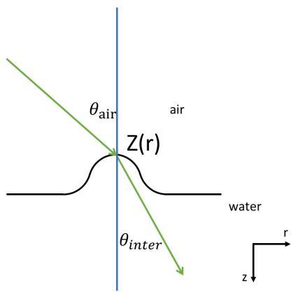
Fig. S11. Display of beam deflection from air-water interface displacement. The origin of the coordinate is the intersection of light and air-water interface.
