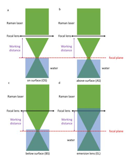
**Fig. S19. Schematics of Raman measurement.** The focal plane is at position of (a) on surface (OS), (b) above surface (AS), (c) below surface (BS), and (d) emersion lens (EL).
