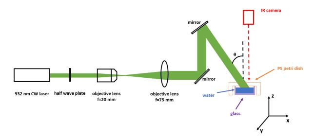
Fig. S24. Optical path for the absorption estimation measurement.
