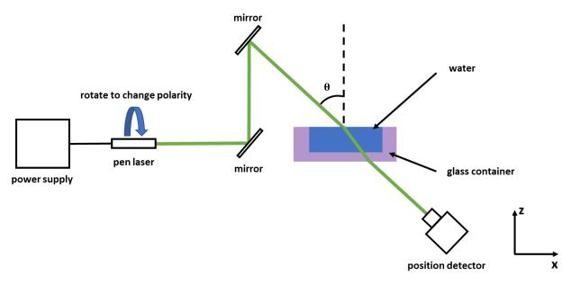
Fig. S8. Optical path of steady-state transmitted beam deflection (SS-TBD) measurement.
