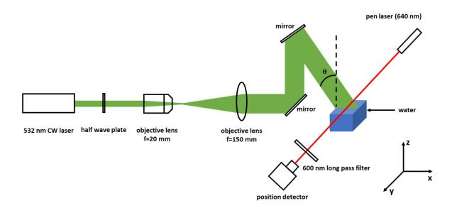
Fig. S6. Optical path of the mirage effect of vapor phase above air-water interface.
