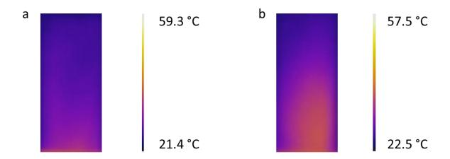
**Fig. S15. IR image of the coverslip above hot water surface.** (a) Under TM-polarized laser illumination (wavelength 532 nm, power 1.4 W, incident angle 45°, 1/e² radius 7.5 mm). The radius of air-water interface is 15 mm. (b) Without laser illumination. Fig. 2g&h plots the temperature distribution along the middle of the coverslip.
