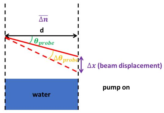
**Fig. S7. Geometry of the measurement of Mirage effect.** Red solid line represents the path of probe light without pump. Red dash line represents the path of probe light with pump on.
