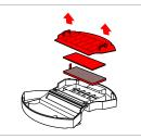
3. Remove the filter cover. then the foam and pleated filters.
