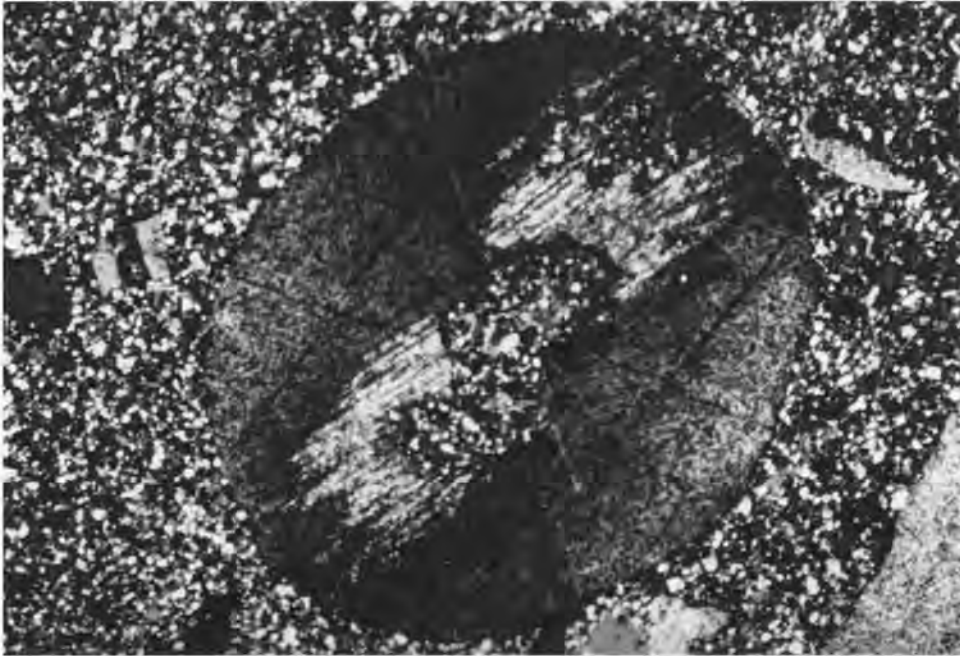
Figure 8.24. Microscope enlargement of a thin rock slice of a deformed crinoid columnal taken from the rock shown in Figure 8.23. The elliptical shape of the crinoid shows the deformation of a fossil that was initially circular in cross section. (This crinoid columnal is about 5 mm in the long direction.)
