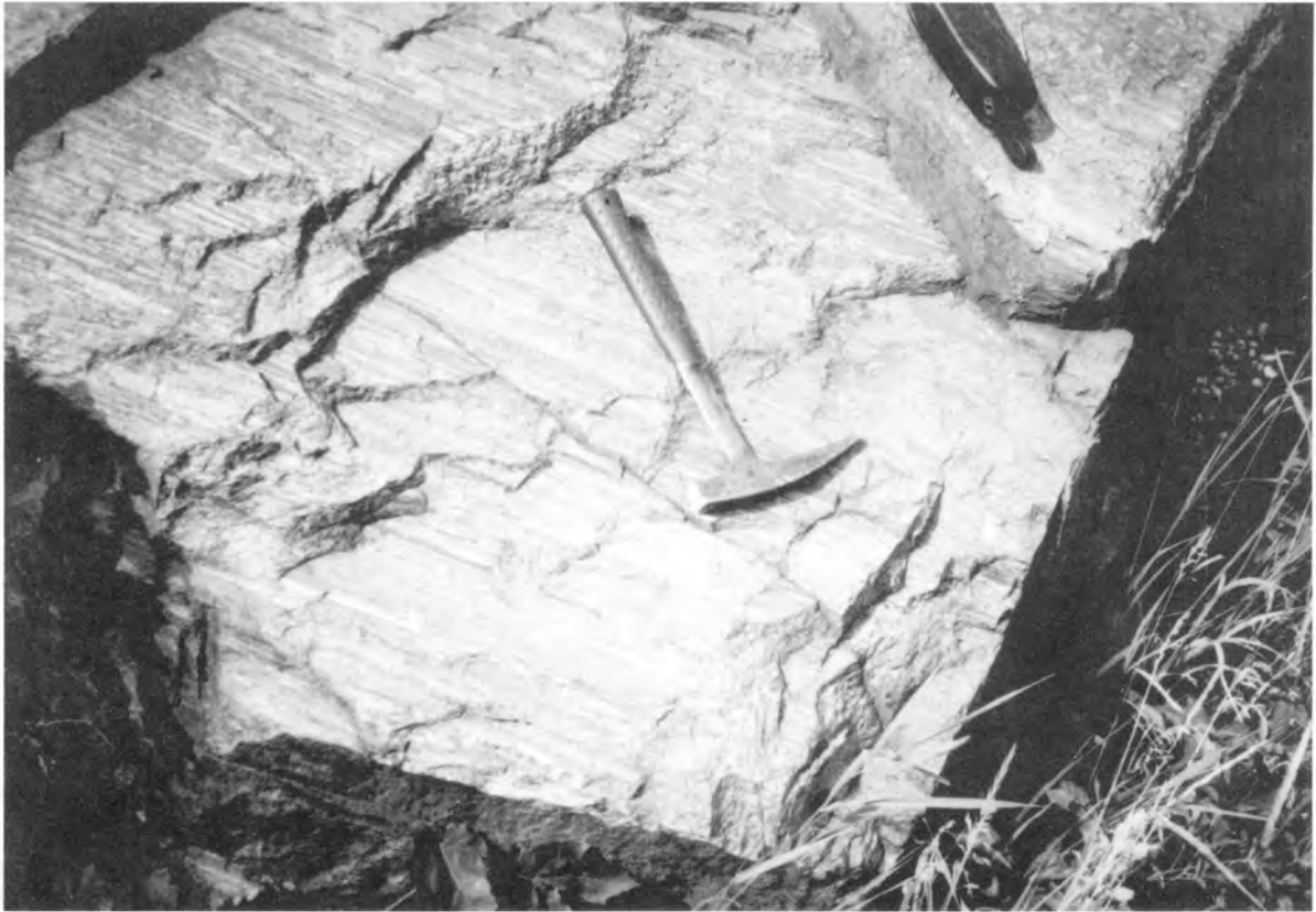
Figure 4.16. This photo shows lineations —streaks of minerals that form in rock when it is severely flattened and stretched. The lineations are ribbon-like bands of quartz; they show the stretching direction. The rock is granitic gneiss.
