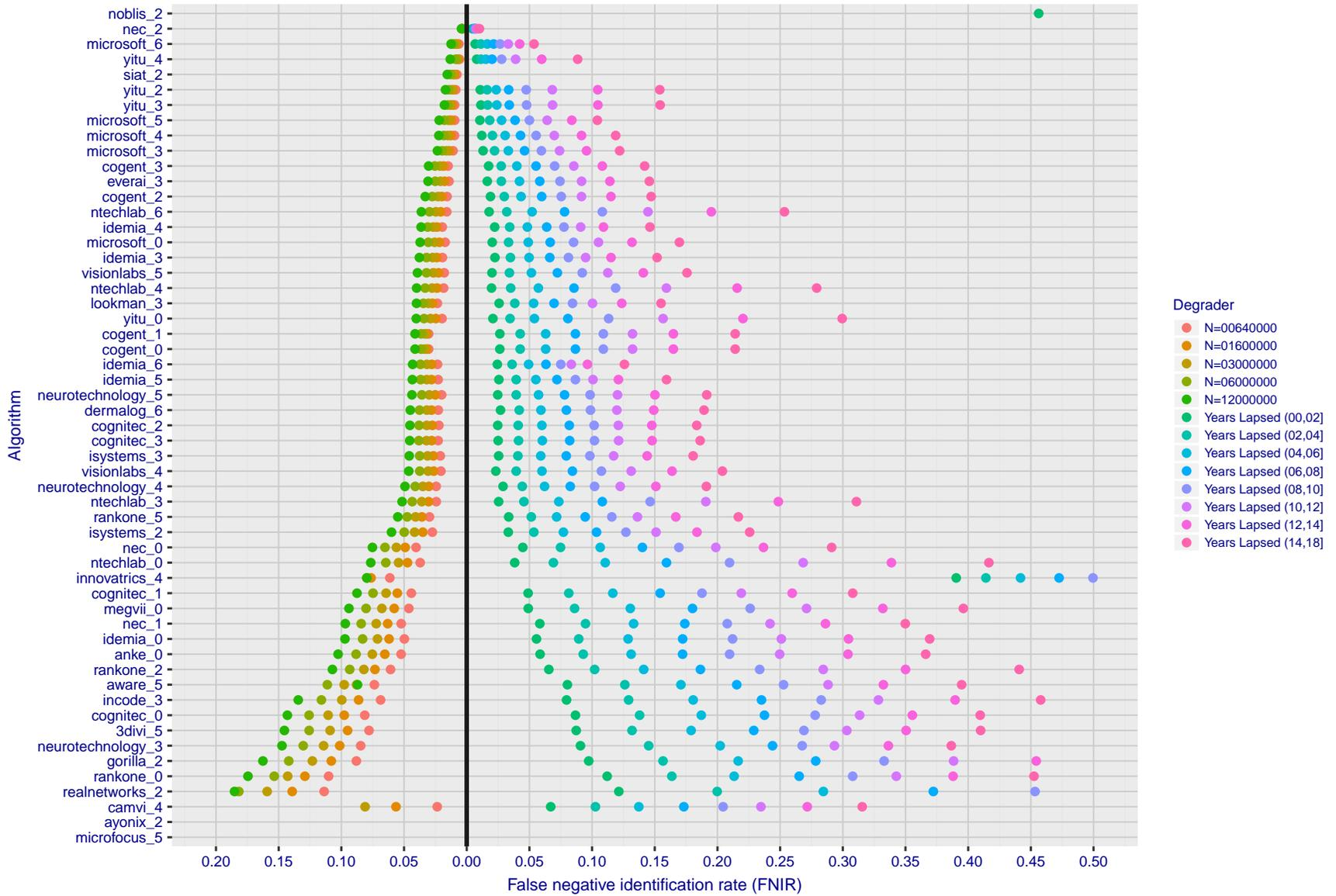
Figure 20: [FRVT-2018 Mugshot Ageing Dataset] Contrast of ageing and population size dependency. The Figure shows, at left, the dependence  $FNIR(N)$  for the FRVT-2018, as tabulated in Table 12. At right, is  $FNIR(N = 3\,000\,000, \Delta T)$  from Figure 62. Ageing miss rates are computed over all searches binned by number of years between search and initial enrollment. In all cases,  $FPIR = 0.01$ .
