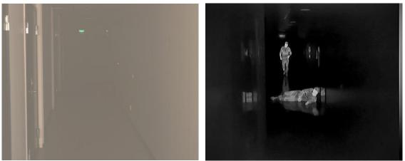
Figure 2: Image taken from a "regular" camera in a smoky hallway (left) and from a thermal network camera (right)
