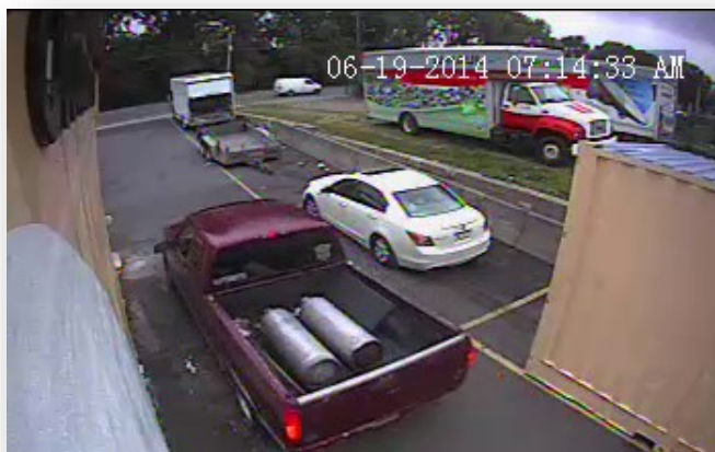
Cylinders filled with propane are at risk of exploding when placed on their sides
